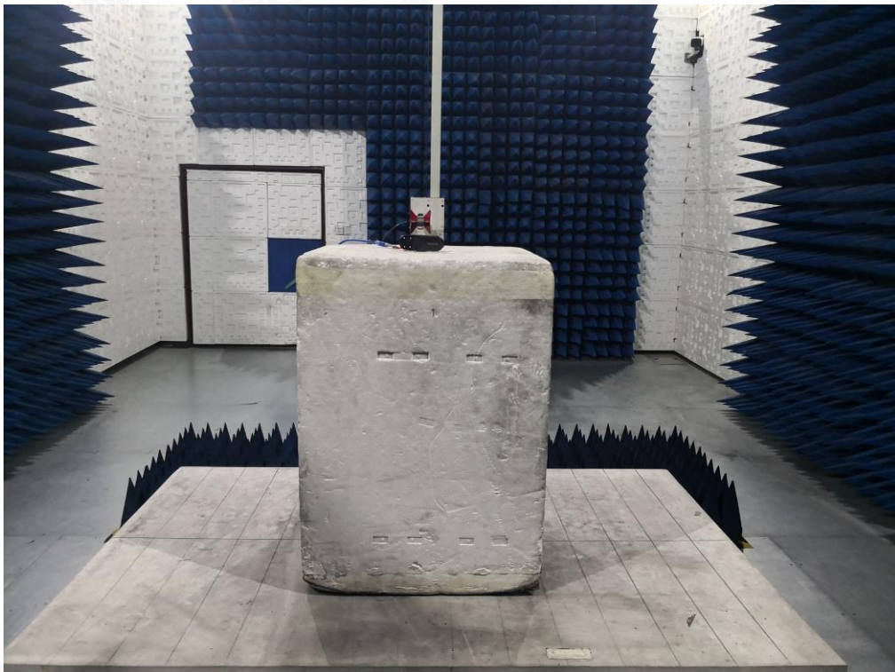
FCC RADIATED EMISSION TEST SETUP ABOVE 1GHZ
