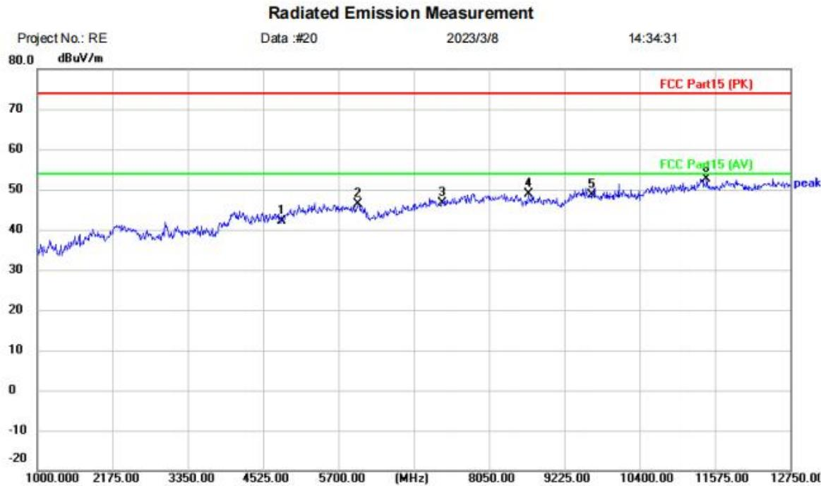
Site: Polarization: **Vertical** Temperature: (C)
