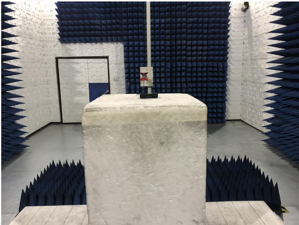
FCC RADIATED EMISSION TEST SETUP ABOVE 1GHZ
