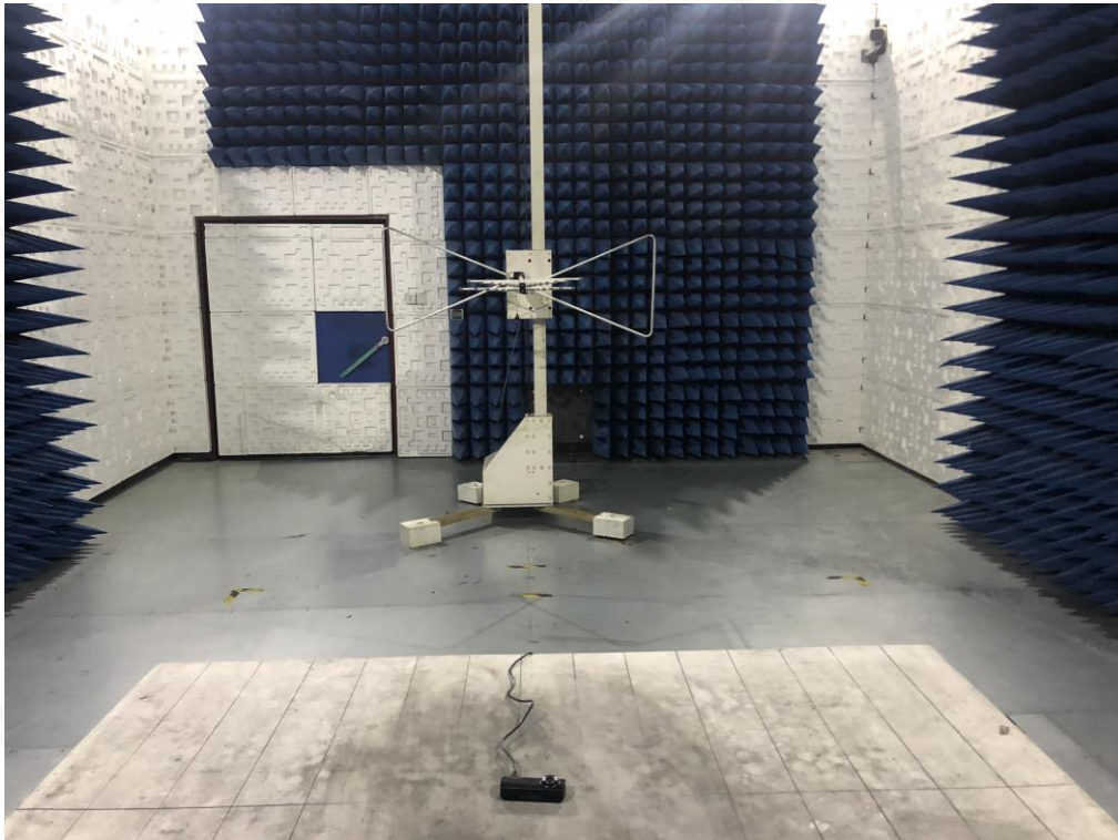
FCC RADIATED EMISSION TEST SETUP ABOVE 1GHZ
