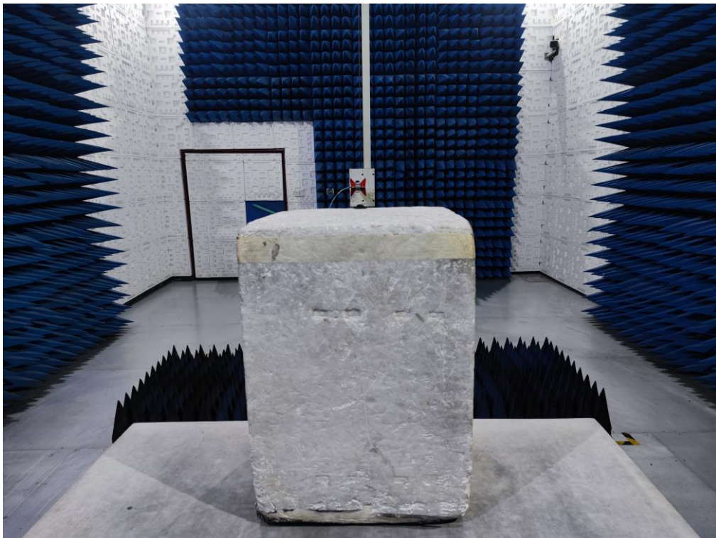
RADIATED EMISSION TEST SETUP ABOVE 1GHZ
