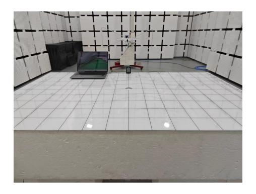
Set-up for Radiated Spurious Emission, Above 1GHz
