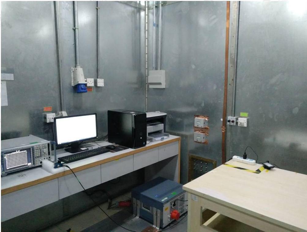
FCC RADIATED EMISSION TEST SETUP BELOW 1GHZ
