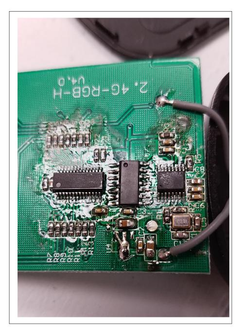
The RF chip installed on the controller, Model # LT8900, is produced by Idctek company. EIKO obtains this chip is through the agency-Shenzhen JMRTH TECh Co. Ltd. under JMRTH's Model #: JMR10P370. For confidential purposes, the identity of the RF chip is masked.
