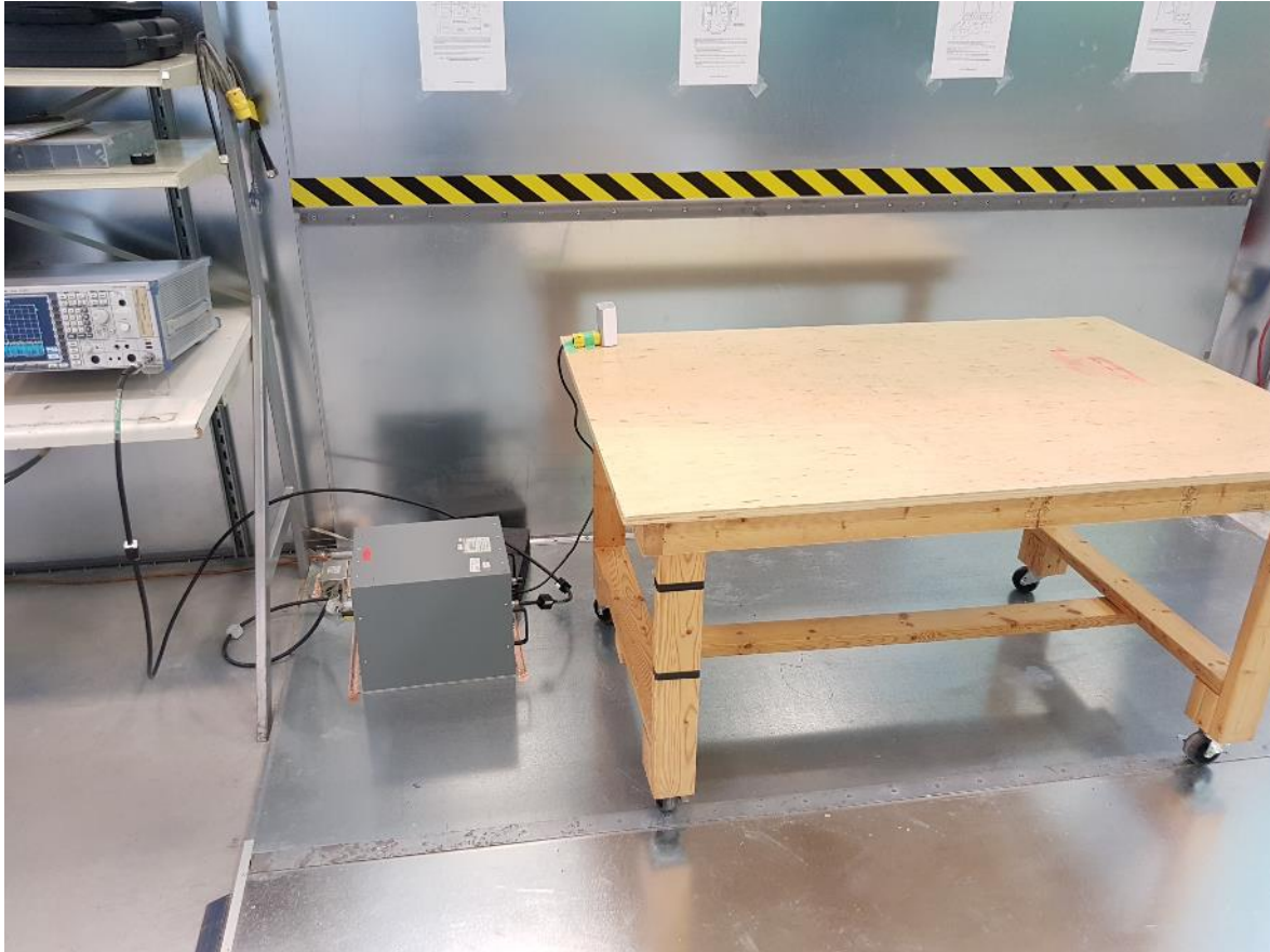
Figure 6 – Conducted Emissions Setup
