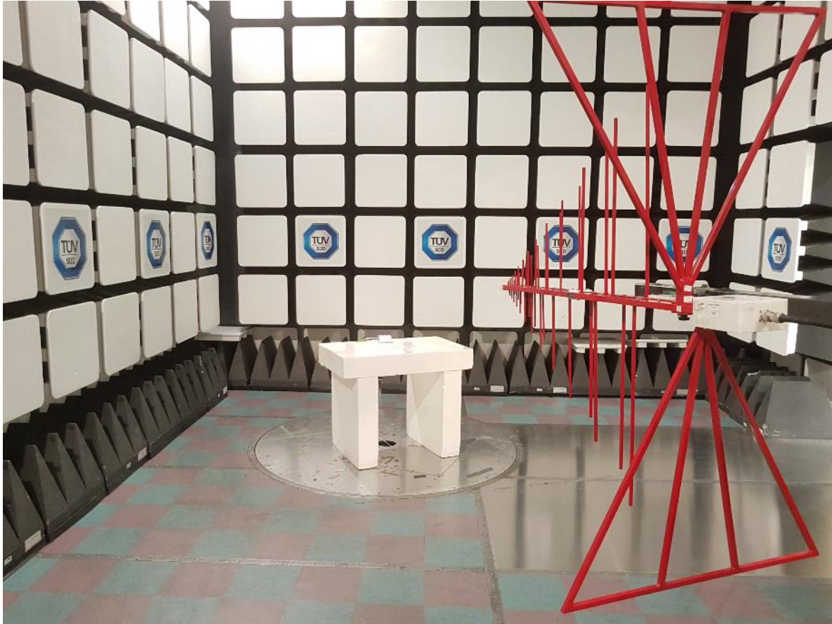
Figure 3 – Radiated Emissions Setup – Photo 2
