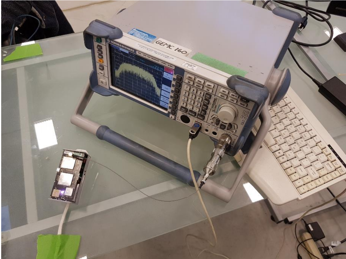
Figure 5 – Antenna Port Conducted Emissions Setup
