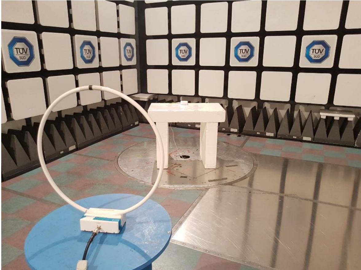
Figure 2 – Radiated Emissions Setup – Photo 1
