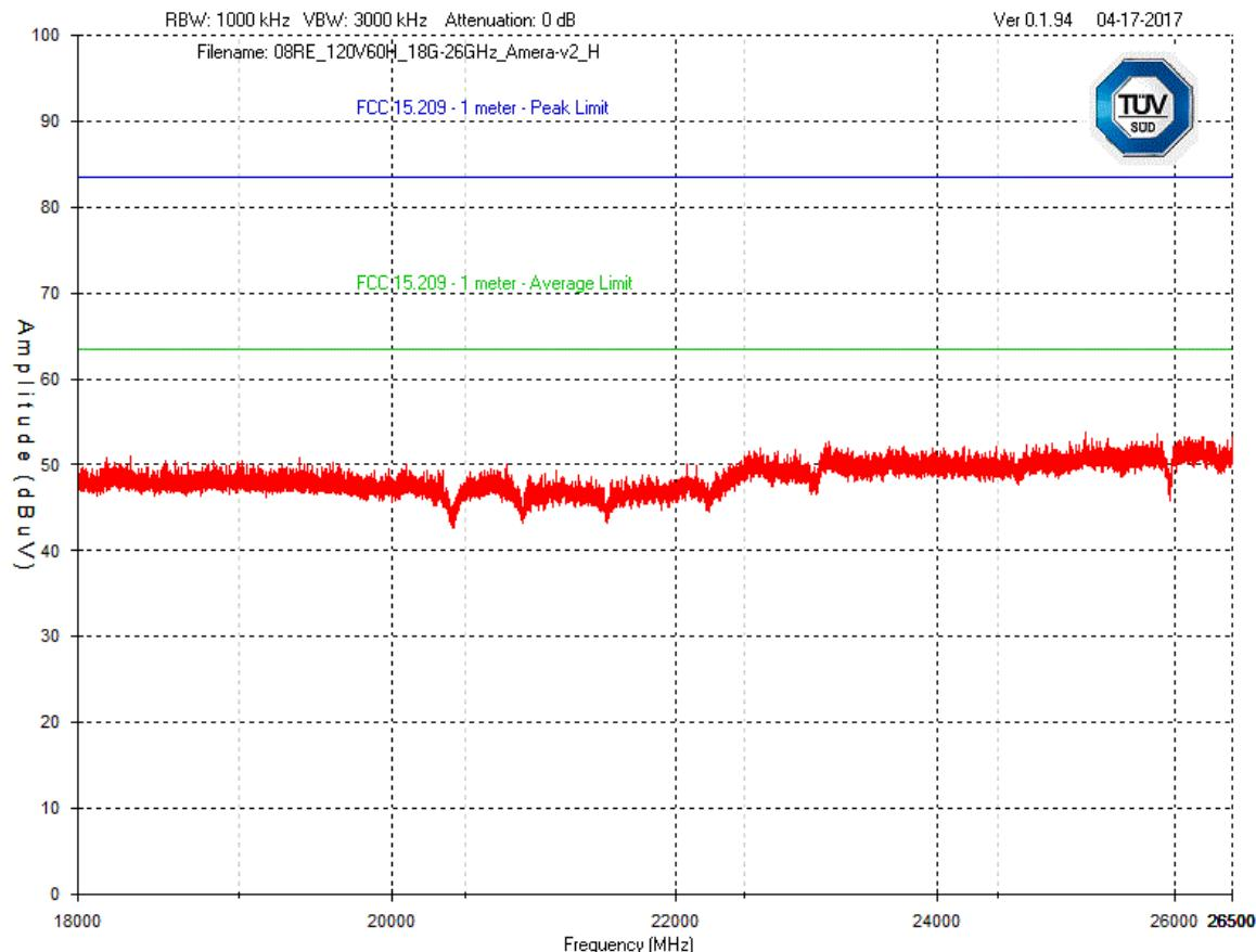
Plot was taken at a 1 meter distance. All emissions were noise floor of measurement instrument. No emissions were found in this frequency range.
