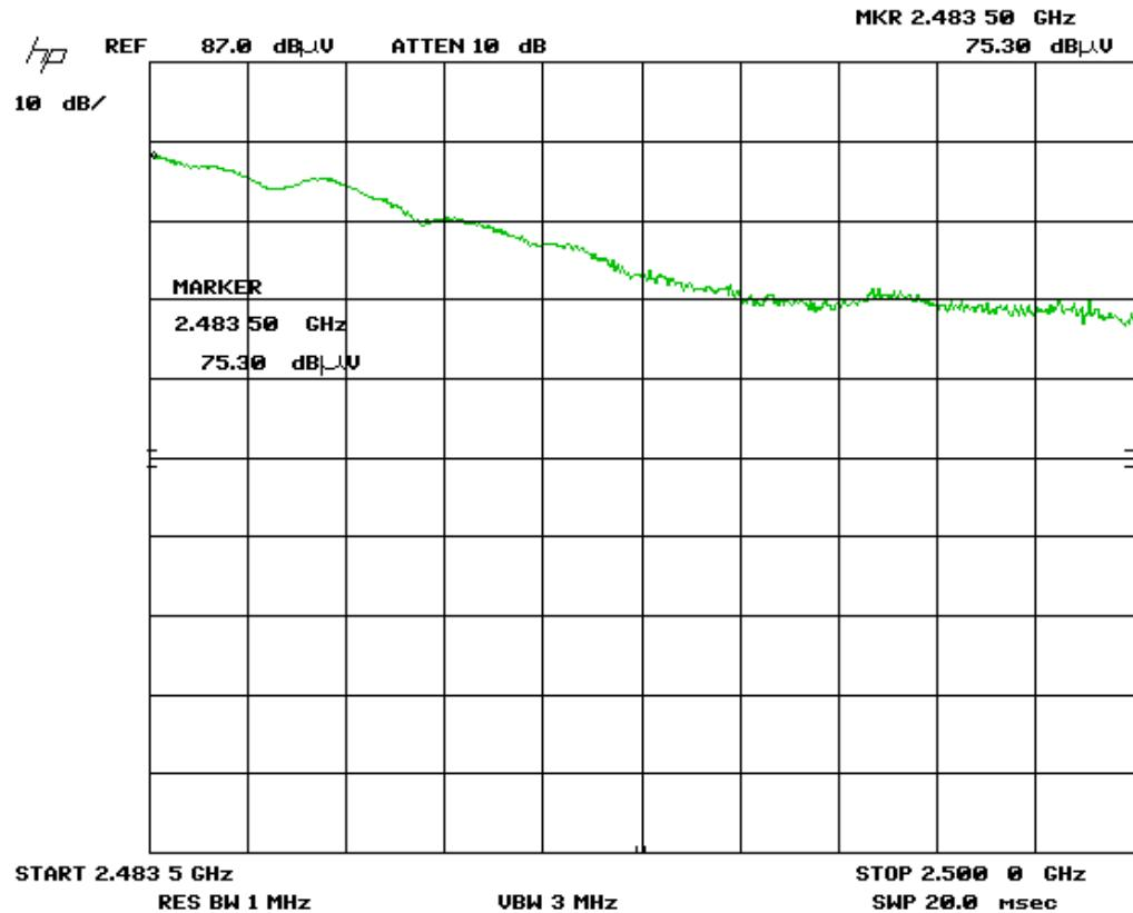
Note: Restricted band Band Edge plot was taken at a 3m measurement distance. The marker shows the raw value. See the Final Measurements and Results section below for correct values.
