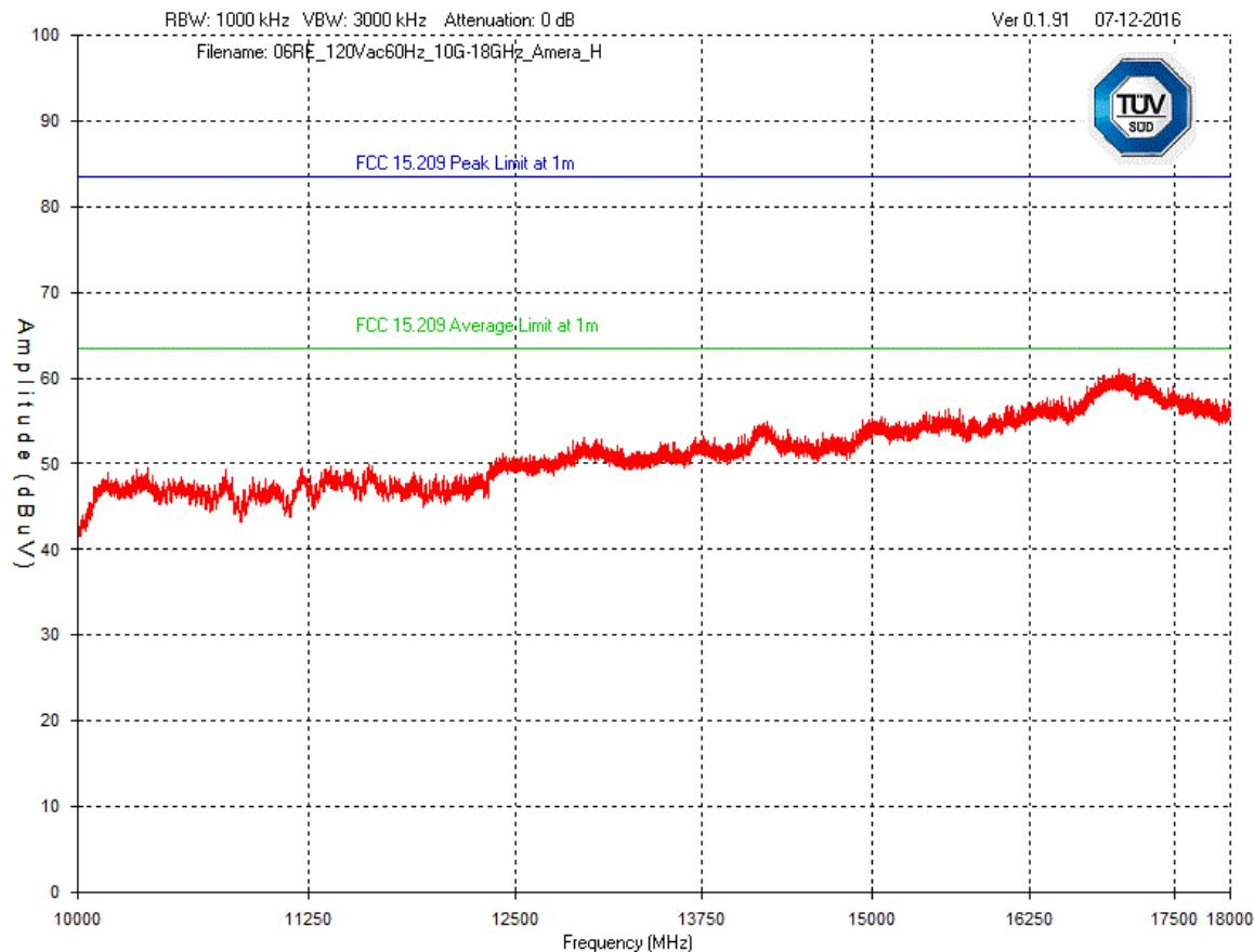
Plot was taken at a 1 meter distance. All emissions were noise floor of measurement instrument. No emissions were found in this frequency range.
