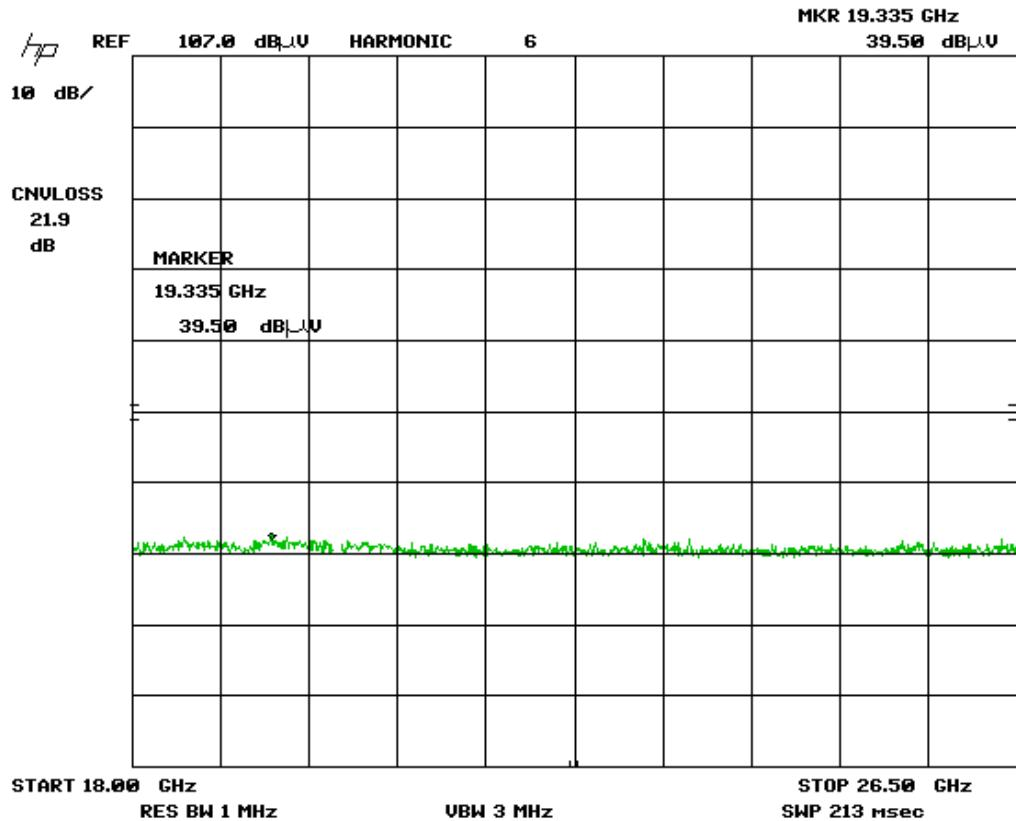
Plot was taken at a 1 meter distance. All emissions were noise floor of measurement instrument. No emissions were found in this frequency range.
