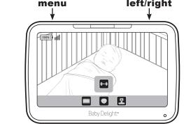
Press the OK button and you should see the PAIRING SCREEN that will appear for 20 seconds.
