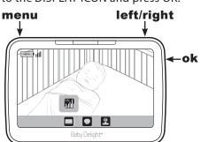
Screen will display TURN MOVEMENT INFO AND ALARM OFF. Use the RIGHT ▶ or LEFT ◀ button to select ON or OFF and press OK.
