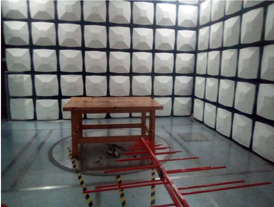
Radiated Emissions View (Below GHz)
