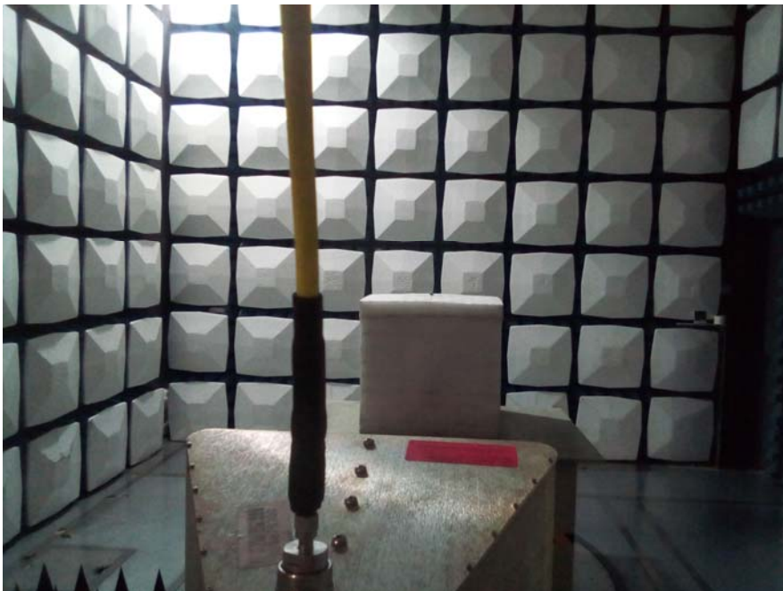
Radiated Emission View (Above 1GHz)
