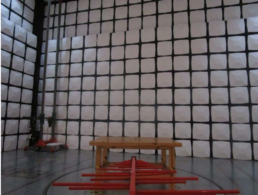
Radiated Emission Transmitting View (Below 1GHz)
