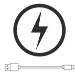
After charging, please pull the charging cable out of the body to avoid the product being charged for a long time. The output voltage and current of the charger is 5V/1A or 5V/1.5A is preferred.If the output voltage and current of the charger exceed the specified, it will cause serious damage to the product, and the product warranty will be invalid at the same time.
