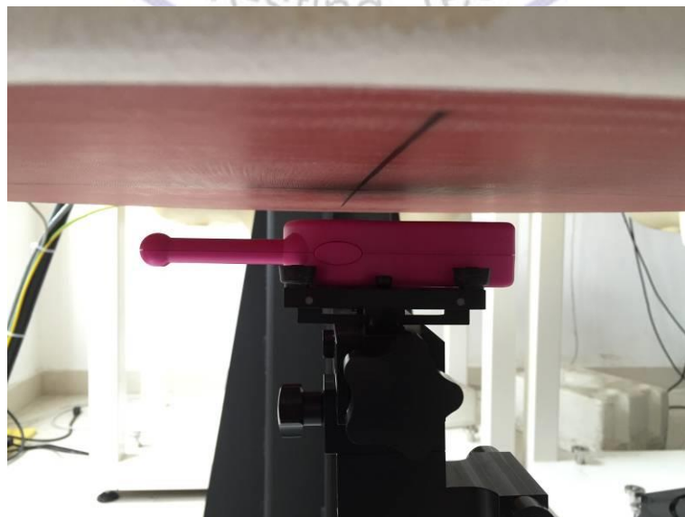
Face-held, the front of the EUT towards phantom (The distance was 25mm between EUT and phantom)
