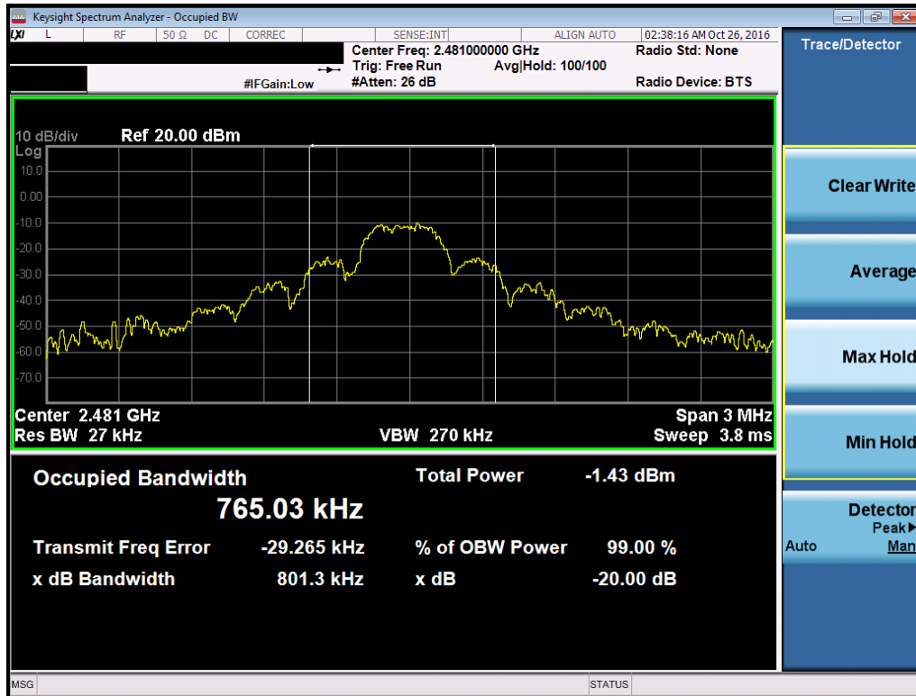
Plot 7-9. 20dB Bandwidth Plot (EX600-WSV3-X41, Ch. 78)
