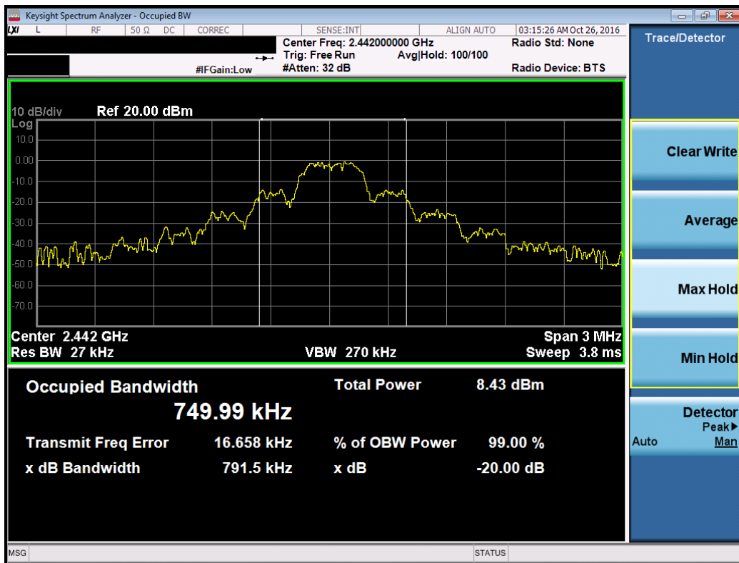
Plot 7-11. 20dB Bandwidth Plot (EX600-WSV4-X41, Ch. 39)
