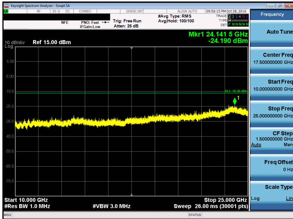
Plot 7-68. Conducted Spurious Plot (EX600-WEN4-X40, Ch. 0)
