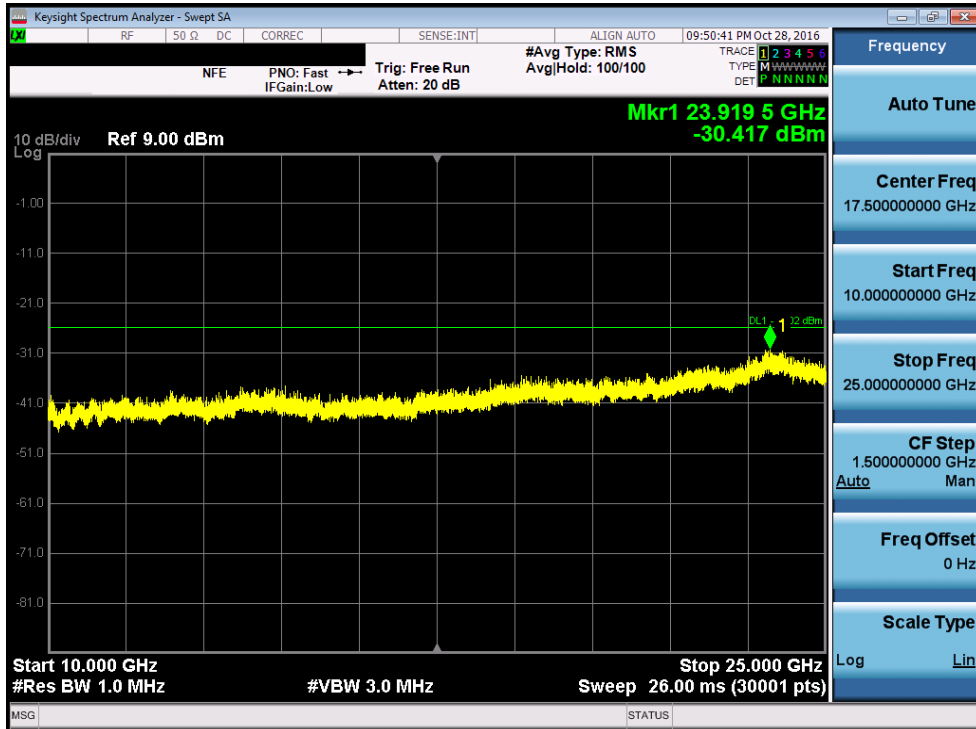
Plot 7-72. Conducted Spurious Plot (EX600-WEN4-X40, Ch. 78)
