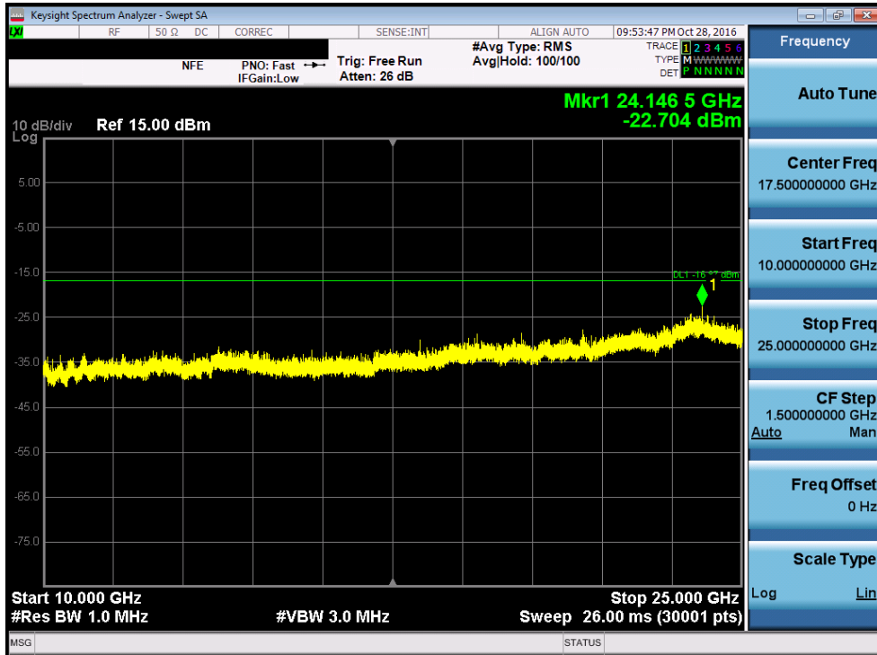
Plot 7-70. Conducted Spurious Plot (EX600-WEN4-X40, Ch. 39)
