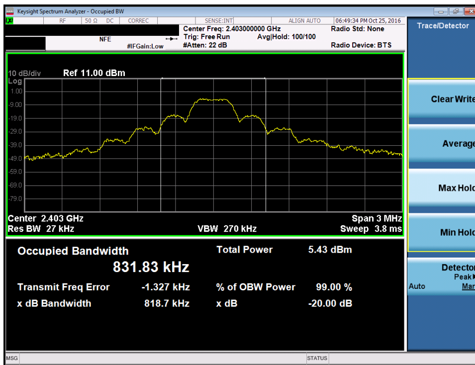
Plot 7-1. 20dB Bandwidth Plot (EX600-WEN3-X40, Ch. 0)
