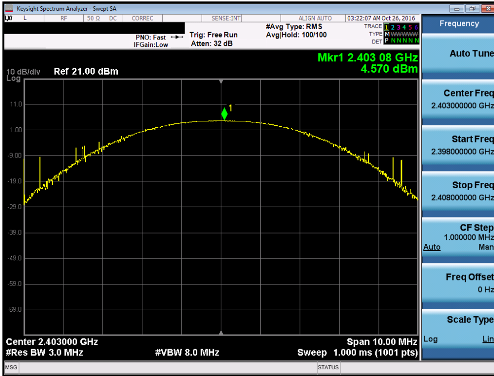
Plot 7-22. Peak Conducted Power (EX600-WSV4-X41, Ch. 0)
