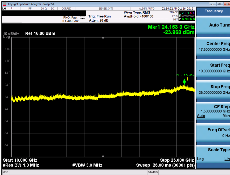
Plot 7-76. Conducted Spurious Plot (EX600-WSV3-X41, Ch. 39)
