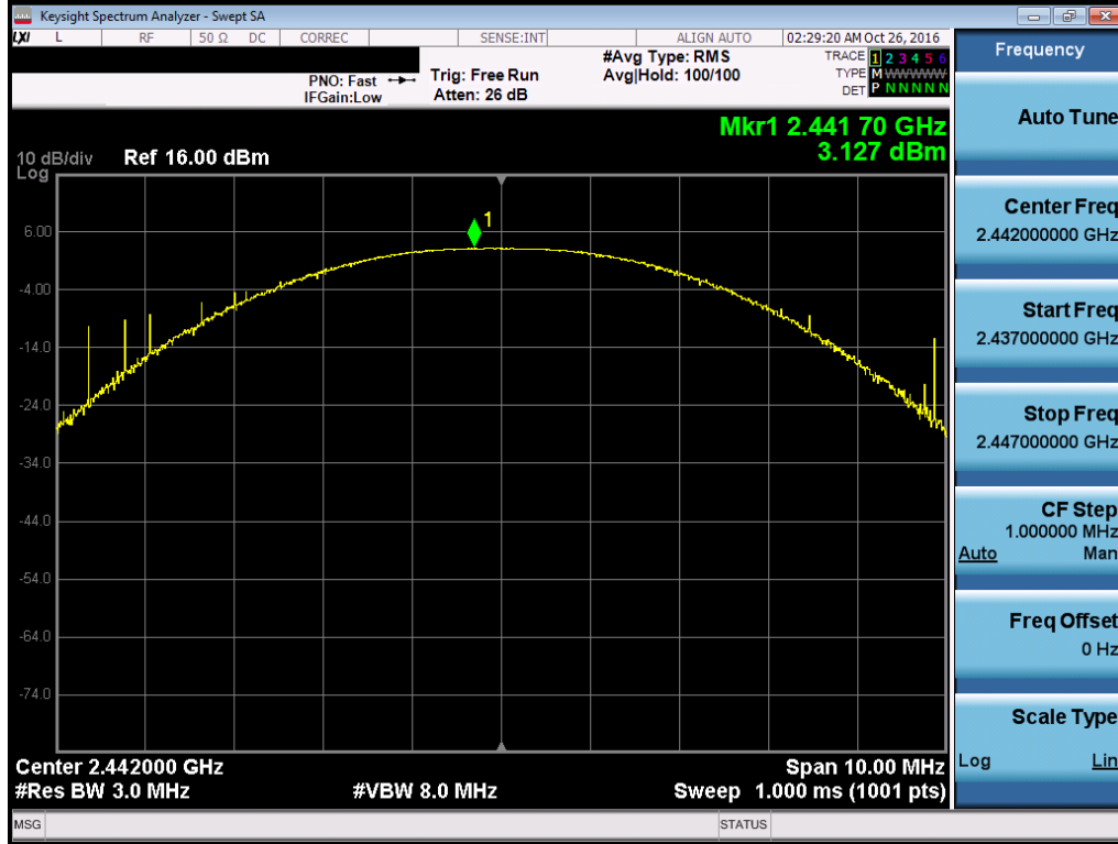
Plot 7-20. Peak Conducted Power (EX600-WSV3-X41, Ch. 39)
