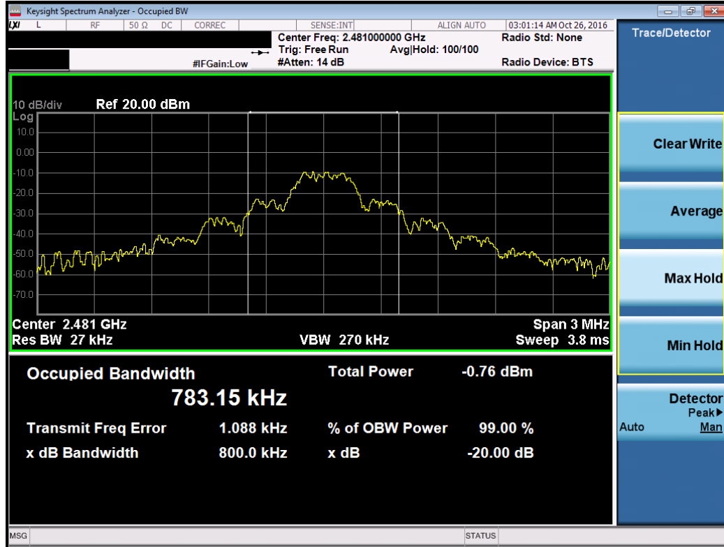
Plot 7-12. 20dB Bandwidth Plot (EX600-WSV4-X41, Ch. 78)
