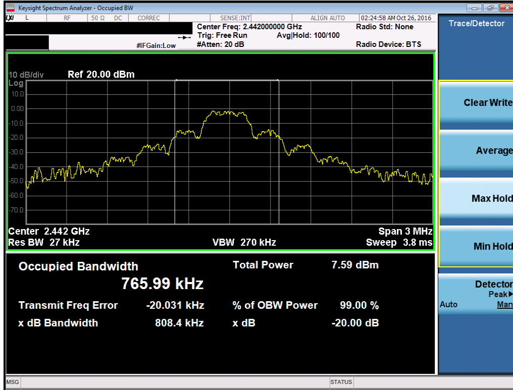
Plot 7-8. 20dB Bandwidth Plot (EX600-WSV3-X41, Ch. 39)
