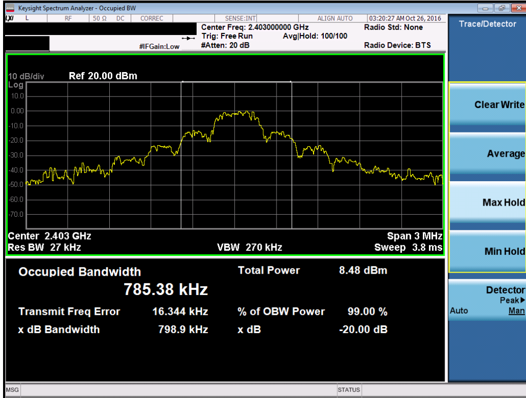
Plot 7-10. 20dB Bandwidth Plot (EX600-WSV4-X41, Ch. 0)
