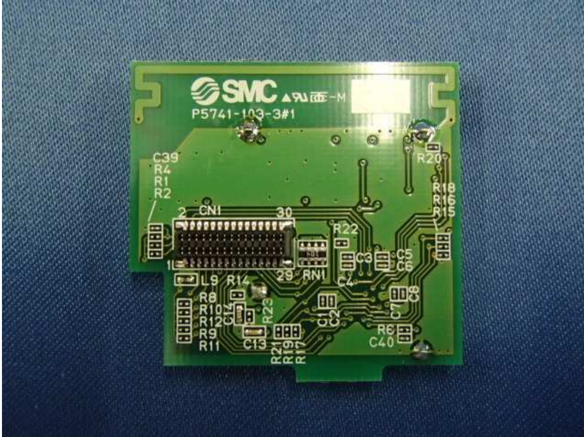
Radio module assembly
