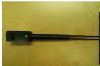
**Figure 1 – MVG COMOSAR Validation Dipole**
