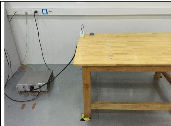
Conducted Emissions Test Setup Front View
