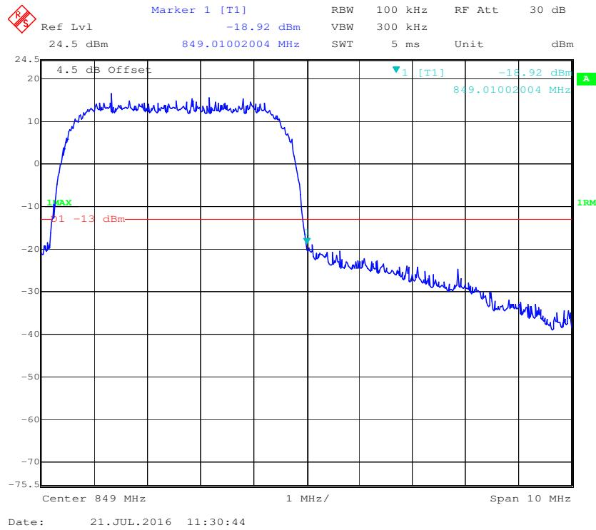
**Cellular Band, Left Band Edge for HSUPA (BPSK) Mode**
