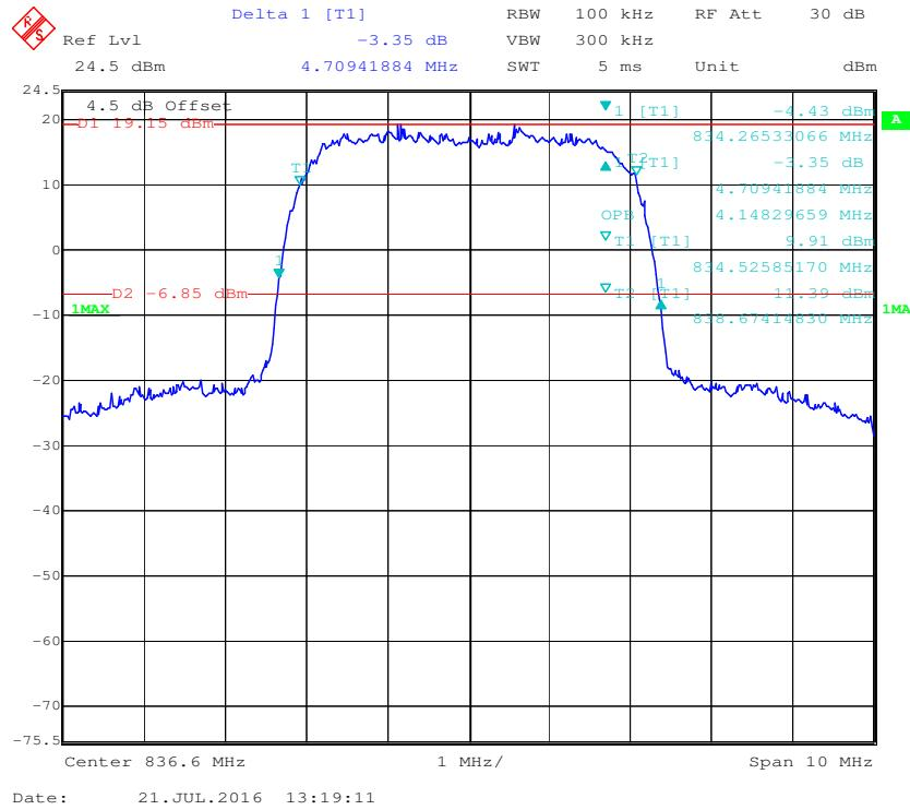
**PCS Band (Part 24E)****99% Occupied & 26 dB Emissions Bandwidth for GSM (GMSK) Mode**
