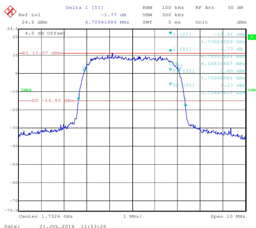
**99% Occupied & 26 dB Emissions Bandwidth for HSDPA (16QAM) Mode**
