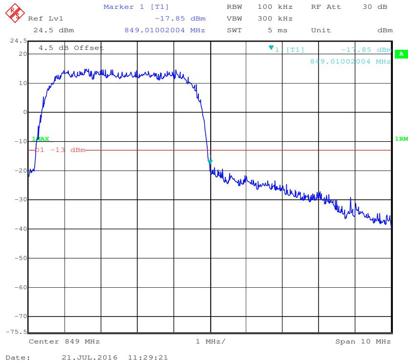
**PCS Band, Left Band Edge for GSM (GMSK) Mode**
