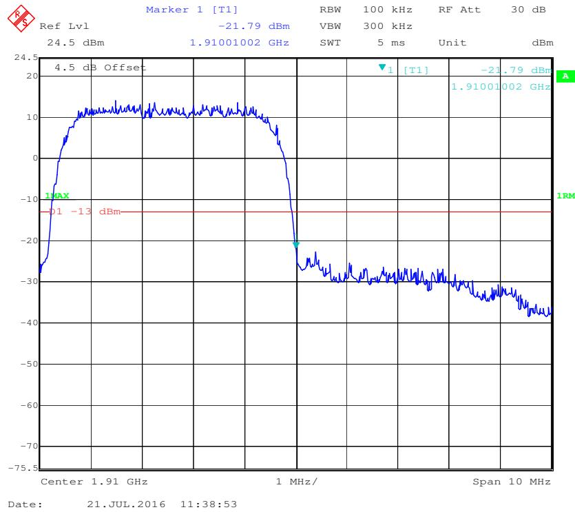
**PCS Band, Left Band Edge for HSUPA (BPSK) Mode**
