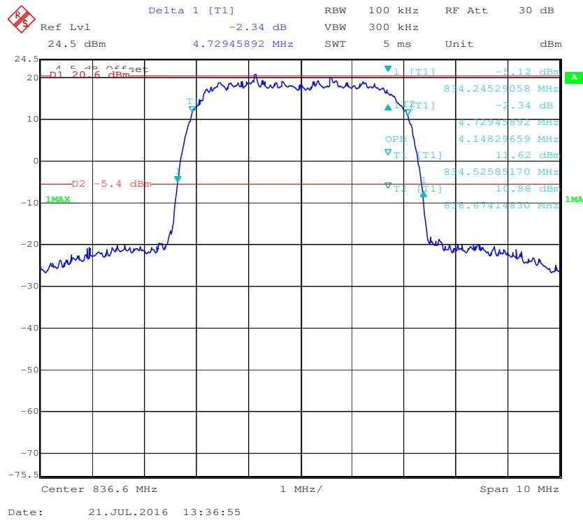
**99% Occupied&26 dB Emissions Bandwidth for HSUPA (BPSK) Mode**
