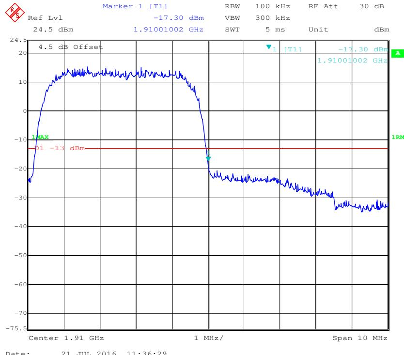
**PCS Band, Left Band Edge for HSDPA (16QAM) Mode**
