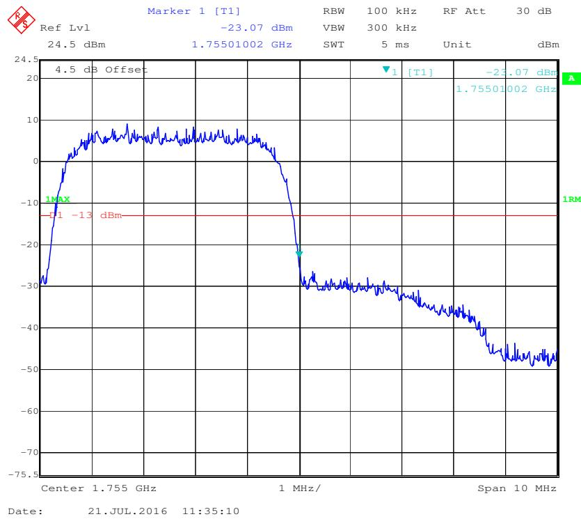
**PCS Band, Left Band Edge for HSDPA (16QAM) Mode**
