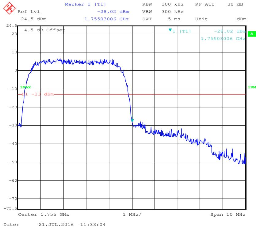
**PCS Band, Left Band Edge for HSUPA (BPSK) Mode**
