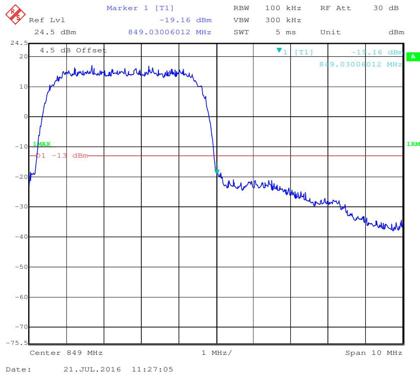
**Cellular Band, Left Band Edge for HSDPA (16QAM) Mode**
