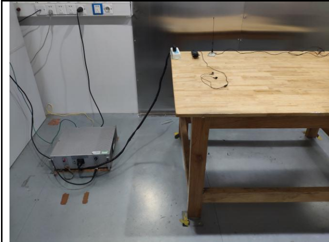
Conducted Emissions Test Setup Front View
