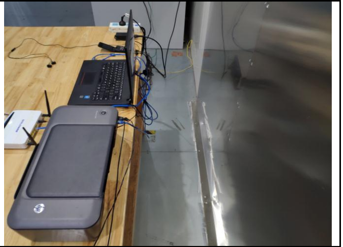
Conducted Emissions Test Setup – Side View
