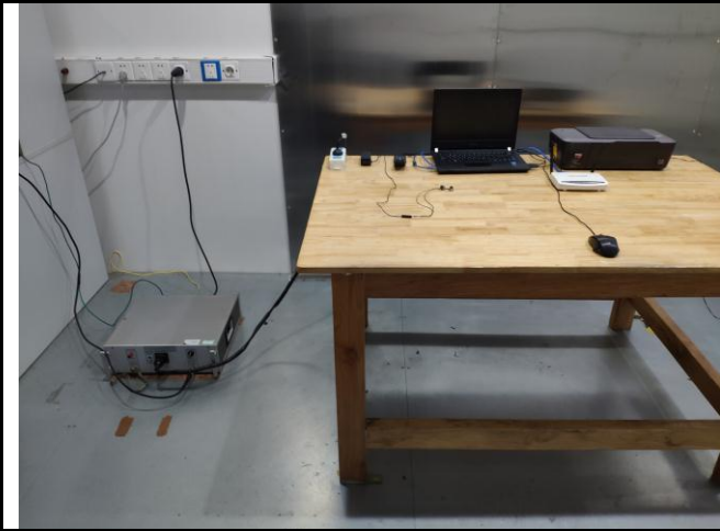
Conducted Emissions Test Setup – Front View
