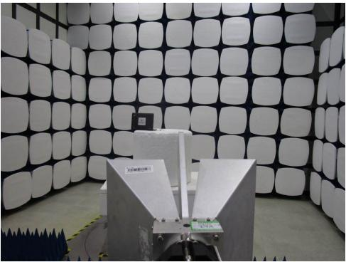
1.2 Radiated Spurious Emissions Test Setup
