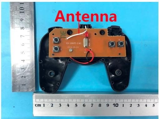
The antenna is integrated on the main PCB and no consideration of replacement. The best case gain of the antenna is 1dBi.
