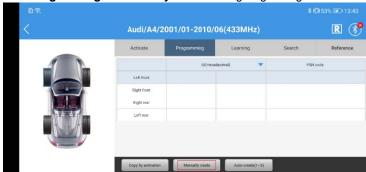
**Note**: Keep the hardware set top close to the new sensor with 10cm.To avoid disturbing, keep other sensors 100cm away from the hardware set.
