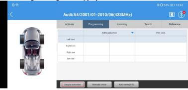
2) If the tip shown as below pops up, you need to activate the original sensor first. Click the **【Ok】** to transfer to the **Activate** interface.
