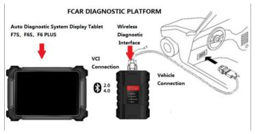
The FCAR diagnostic platform combines the VCI device and the display tablet with technical information into ensuring quick and simple access to the vehicle to perform comprehensive diagnostics applications.
