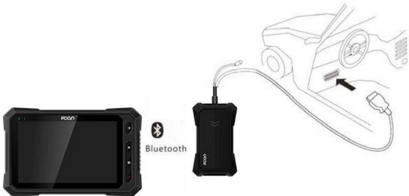
Figure 3.2-1 Connection of standard-OBD-II port
