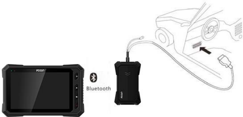
Figure 3.2-1 Connection of standard-OBD-II port
