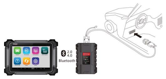
Then turn on the machine, enter [Settings]-[VCI connection]. It can be connected via Bluetooth and USB cable:
