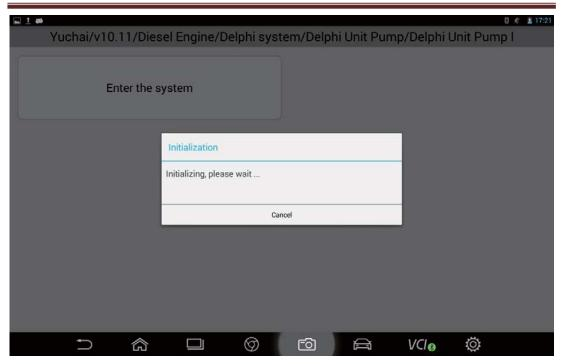
8. After that, Read ECU Information, Read Fault code, Erase Fault Code, Read Data Stream can be seen.
