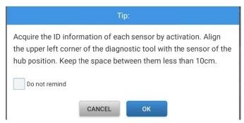
**Note**: Keep the hardware set top close to the sensor **to be programed** with 10cm. To avoid disturbing, keep other sensors100cm away from the hardware set.
