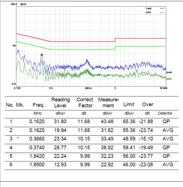
Remark: Factor = LISN factor + Cable Loss + Pulse limiter factor.
