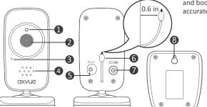
Keep the distance between sensor and body at least 0.6 inch for accurate temperature result.
