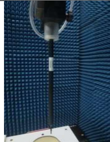
Fig. 8.2 Photo of E-Field Probe
