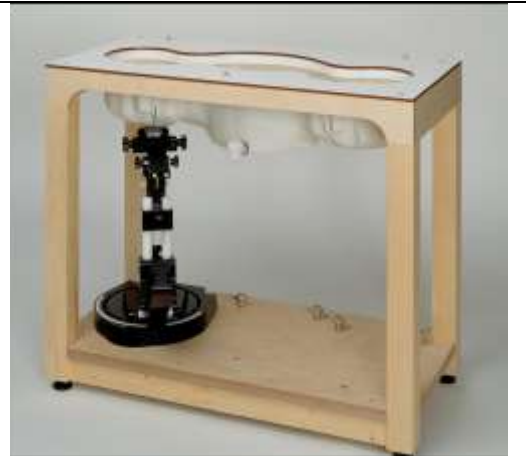
Fig. 8.7 Photo of SAM Twin Phantom
