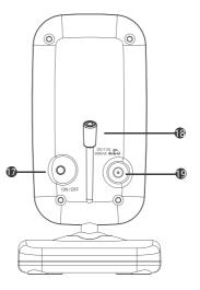
13 Nighttime LEDs 14 Lens 15 Microphone 16 Speaker 17 Power On / Off Switch 18 Temperature sensor 19 DC Jack
