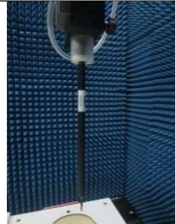
Fig. 8.2 Photo of E-Field Probe
