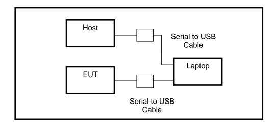
Note: The Host and the EUT are identical BLE device, the engineering mode need two BLE device work together.
