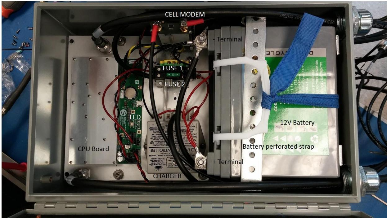
The Interrogator box contains a baseplate with all electronics and a battery.
