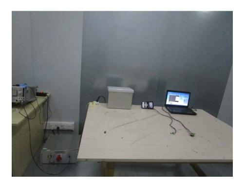
Radiation Emission Test Setup (Below 30MHz)
