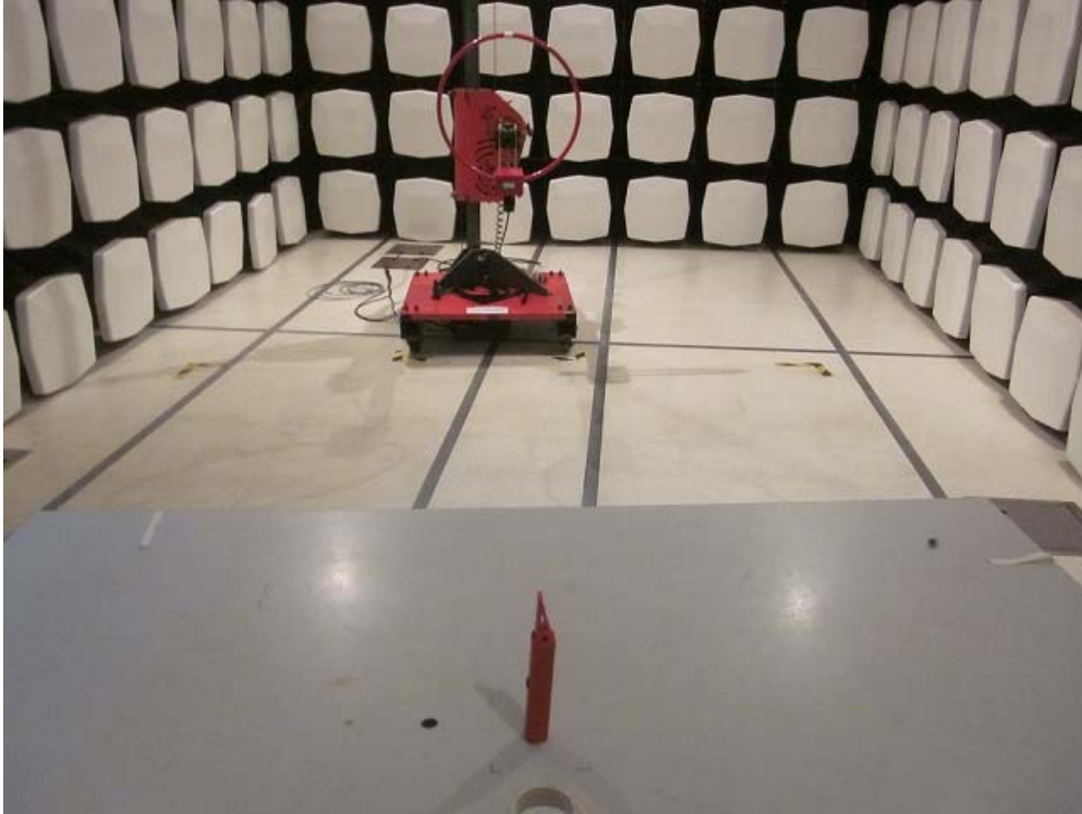
Measurement of Radiated Emission Test Set Up
