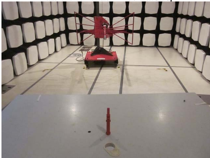
Measurement of Radiated Emission Test Set Up
