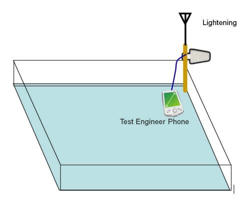
Fix the donor antenna after selecting the best position, and adjust slightly its height or angles in order to get the signals with suitable input power level and calling quality.
