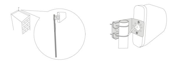
■ Installation of YAGI antenna as donor antenna
