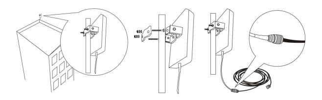
■ Installation of wide directional antenna as donor antenna
