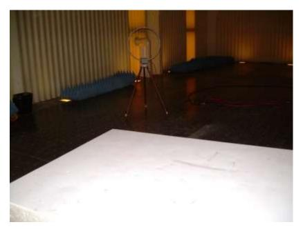
Photograph 12: Reference Photo of Test Setup for Emissions Below 30 MHz
