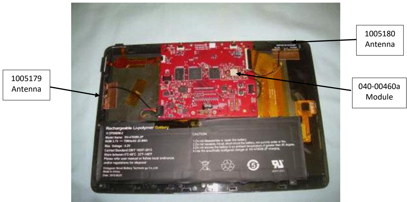
Photograph 4 – Internal View, C4-T4T10
