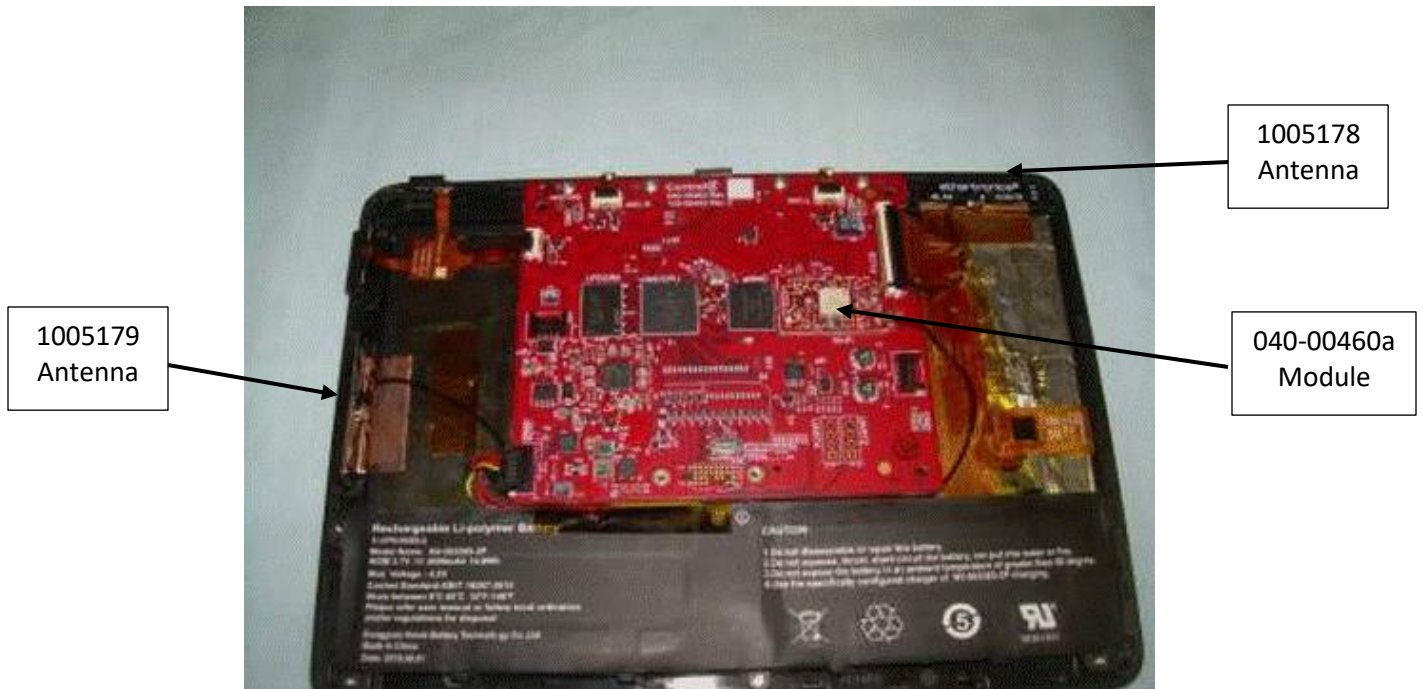
Photograph 3 – Internal View, C4-T4T8
