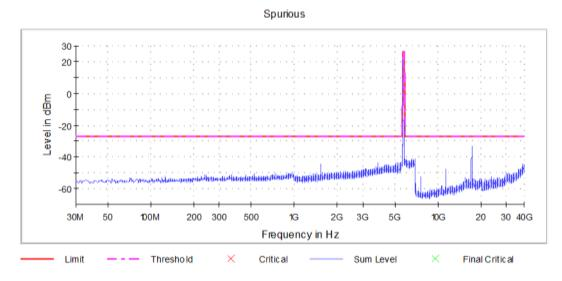
Graph 29: Antenna 1 – Spurious Emissions Channel 149 Transmitting (5745 MHz) - Setting 20
