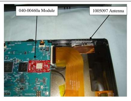
Photograph 21: 040-00460a Installed in C4-T4IW10-XX with 1005097 Antenna Installed
