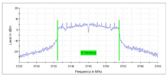
Graph 11: Antenna 1 - 6 dB Emissions Bandwidth Transmitting at 5745 MHz - Setting 20
