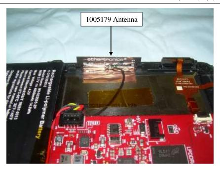
Photograph 19: 040-00460a Installed in C4-T4T8-XX with 1005179 Antenna Installed
