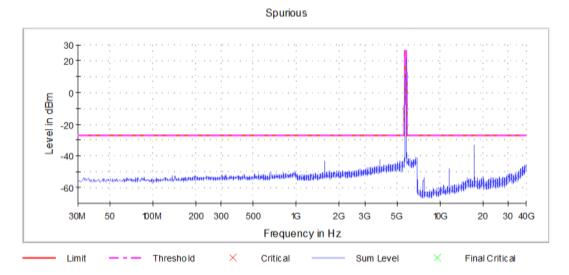
Graph 30: Antenna 1 – Spurious Emissions Channel 157 Transmitting (5785 MHz) - Setting 20
