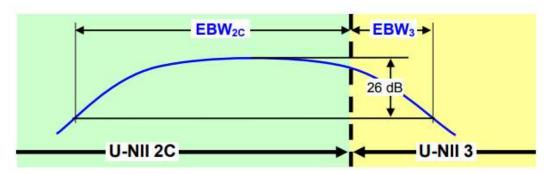
Figure 5. Non-overlapping emissions bandwidths (KDB 789033 D02 v02r01, p 19)
