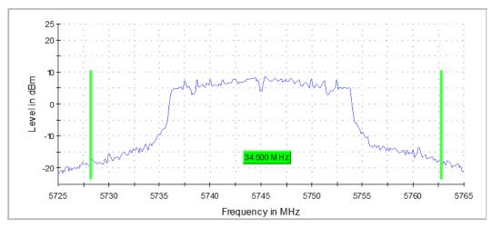
Graph 5: Antenna 1 – 26 dB Emissions Bandwidth Transmitting at 5745 MHz – Setting 20
