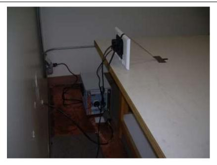
Photograph 11 – Back View Conducted Emissions Configuration – In-wall Units AC Powered
