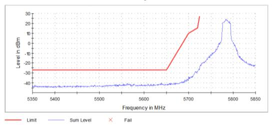
Graph 22: Antenna 1 – Lower Band Edge Channel 157 Transmitting (5785 MHz) - Setting 20
