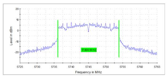
Graph 8: Antenna 0 – 6 dB Emissions Bandwidth Transmitting at 5745 MHz - Setting 20
