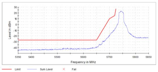
Graph 20: Antenna 1 – Lower Band Edge Channel 149 Transmitting (5745 MHz) - Setting 20
