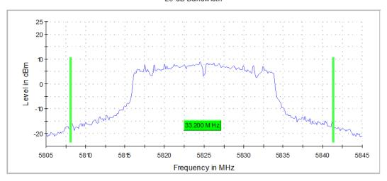
Graph 4: Antenna 0 – 26 dB Emissions Bandwidth Transmitting at 5825 MHz – Setting 20
