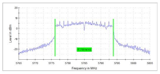
Graph 9: Antenna  $0-6\ dB$  Emissions Bandwidth Transmitting at 5785 MHz - Setting 20
