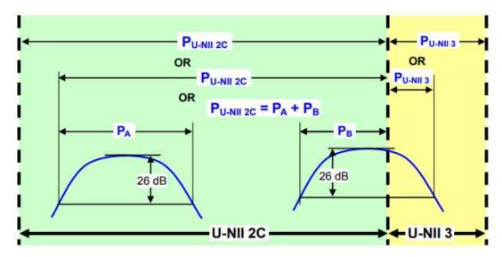
Figure 2. Conducted output power measurement examples (KDB 789033 D02 v02r01, p 21)
