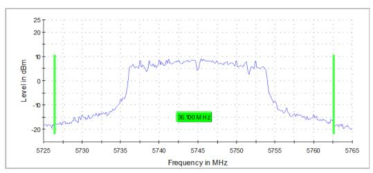
Graph 2: Antenna 0 – 26 dB Emissions Bandwidth Transmitting at 5745 MHz – Setting 20
