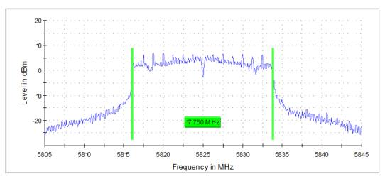
Graph 10: Antenna  $0-6\ dB$  Emissions Bandwidth Transmitting at 5825 MHz - Setting 20
