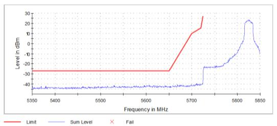
Graph 18: Antenna 0 – Lower Band Edge Channel 165 Transmitting (5825 MHz) - Setting 20
