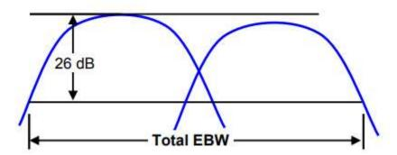
Figure 3. Overlapping emissions bandwidths (KDB 789033 D02 v02r01, p 18)
