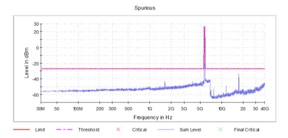
Graph 31: Antenna 1 – Spurious Emissions Channel 165 Transmitting (5825 MHz) - Setting 20
