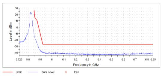
Graph 25: Antenna 1 – Upper Band Edge Channel 165 Transmitting (5825 MHz) - Setting 20
