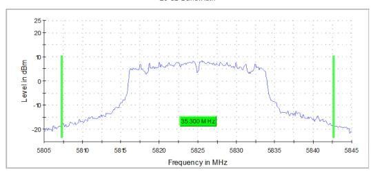
Graph 7: Antenna 1 – 26 dB Emissions Bandwidth Transmitting at 5825 MHz – Setting 20
