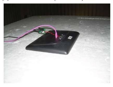
Photograph 6: Back Radiated Emissions Configuration – Tabletop Unit Horizontal Placement
