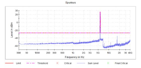
Graph 26: Antenna 0 – Spurious Emissions Channel 149 Transmitting (5745 MHz) - Setting 20
