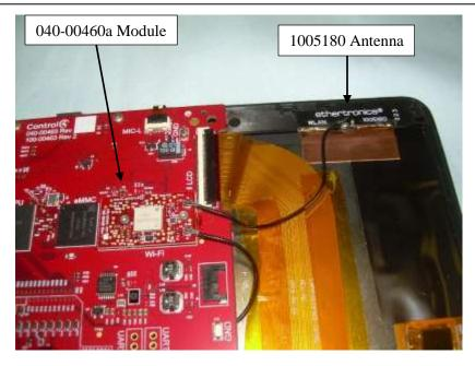
Photograph 15: 040-00460a Installed in C4-T4T10-xxwith 1005180 Antennas Installed
