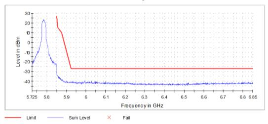
Graph 23: Antenna 1 – Upper Band Edge Channel 157 Transmitting (5785 MHz) - Setting 20
