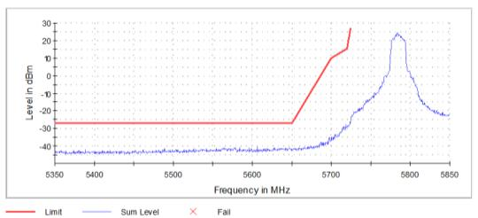
Graph 16: Antenna 0 - Lower Band Edge Channel 157 Transmitting (5785 MHz) - Setting 20
