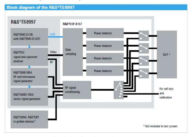
Figure 2: Direct Connection at the Antenna Port Test
