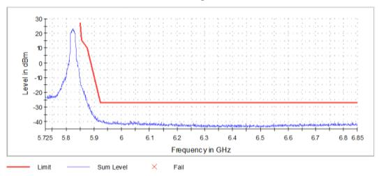
Graph 19: Antenna 0 – Upper Band Edge Channel 165 Transmitting (5825 MHz) - Setting 20
