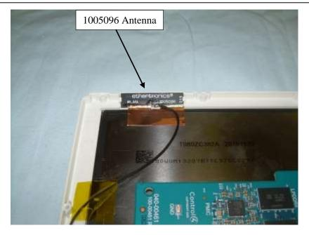
Photograph 25: 040-00460a Installed in C4-T4IW8-XX with 1005096 Antenna Installed
