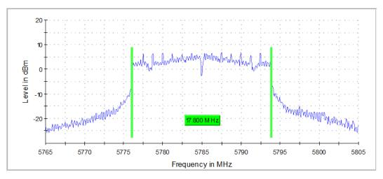
Graph 12: Antenna  $1-6\ dB$  Emissions Bandwidth Transmitting at 5785 MHz - Setting 20
