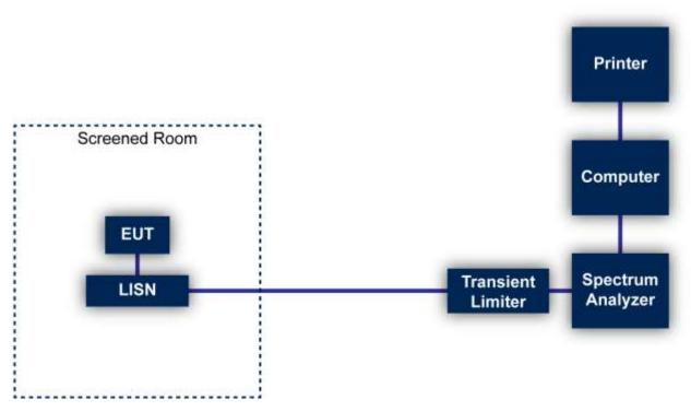
**Figure 1: Mains Conducted Emissions Test**
