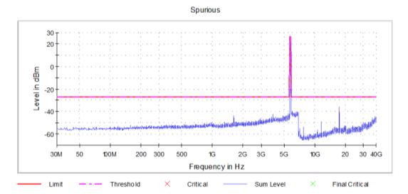
Graph 28: Antenna 0 – Spurious Emissions Channel 165 Transmitting (5825 MHz) - Setting 20 Antenna 1 Spurious Domain Measurements
