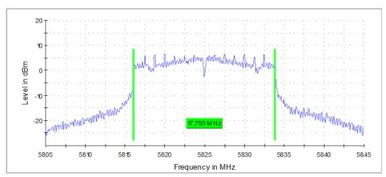
Graph 13: Antenna 1 - 6 dB Emissions Bandwidth Transmitting at 5825 MHz - Setting 20
