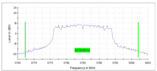
Graph 3: Antenna 0 - - 26 dB Emissions Bandwidth Transmitting at 5785 MHz - Setting 20
