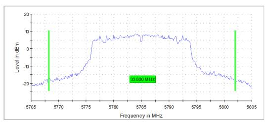
Graph 6: Antenna 1 – 26 dB Emissions Bandwidth Transmitting at 5785 MHz – Setting 20
