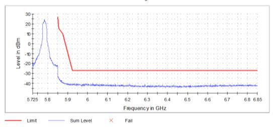
Graph 17: Antenna 0 – Upper Band Edge Channel 157 Transmitting (5785 MHz) - Setting 20
