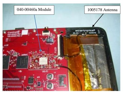
Photograph 18: 040-00460a Installed in C4-T4T8-XX with 1005178 Antenna Installed
