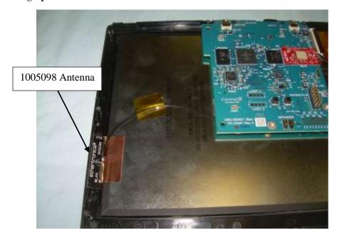
Photograph 22: 040-00460a Installed in C4-T4IW10-XX with 1005098 Antenna Installed
