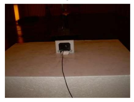
Photograph 4: Back View Radiated Emissions Configuration – Above 1000 MHz – C4-T4IW10-XX Shown
