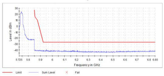
Graph 21: Antenna 1 – Upper Band Edge Channel 149 Transmitting (5745 MHz) - Setting 20
