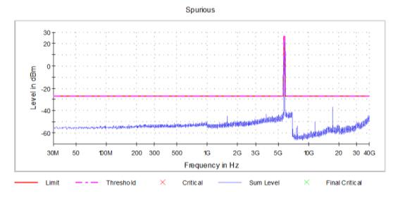
Graph 27: Antenna 0 – Spurious Emissions Channel 157 Transmitting (5785 MHz) - Setting 20
