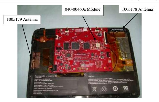
Photograph 17: 040-00460a Installed in C4-T4T8-XX with 1005178 and 1005179 Antennas Installed
