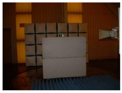
Photograph 3: Front View Radiated Emissions Configuration – Above 1000 MHz – C4-T4IW10-XX Shown
