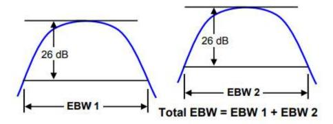
Figure 4. Non-overlapping emissions bandwidths (KDB 789033 D02 v02r01, p 18)
