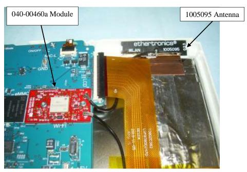
Photograph 24: 040-00460a Installed in C4-T4IW8-XX with 1005095 Antennas Installed
