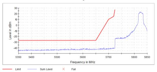
Graph 24: Antenna 1 – Lower Band Edge Channel 165 Transmitting (5825 MHz) - Setting 20
