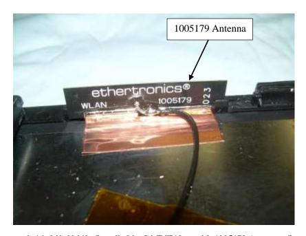
Photograph 16: 040-00460a Installed in C4-T4T10-xxwith 1005179 Antennas Installed
