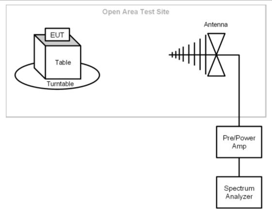
Figure 3: Radiated Emissions Below 1GHz Test
