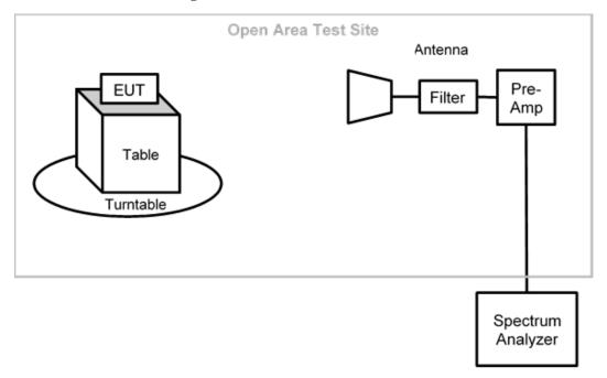
Figure 4: Radiated Emissions Above 1GHz Test
