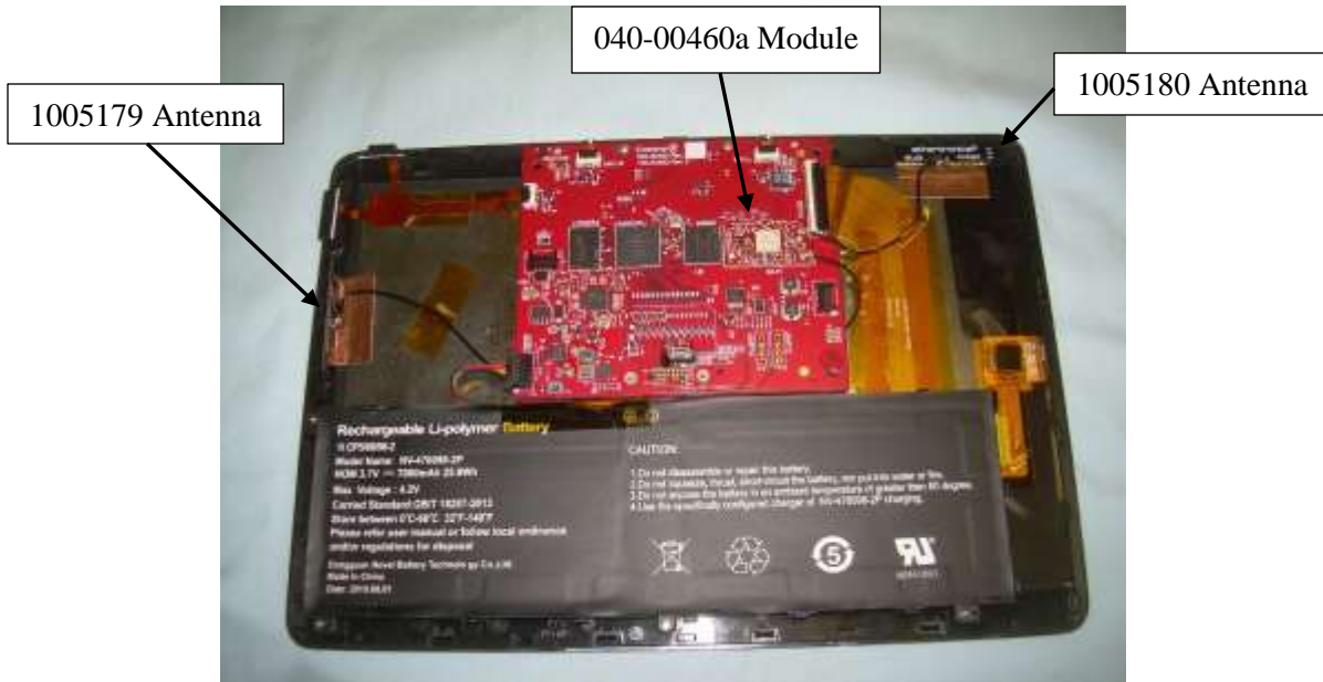
Photograph 14: 040-00460a Installed in C4-T4T10-xx with 1005180 and 1005179 Antennas Installed
