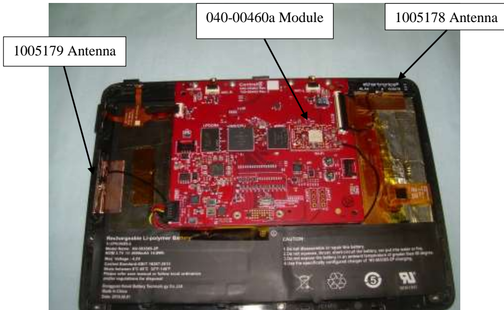
Photograph 17: 040-00460a Installed in C4-T4T8-XX with 1005178 and 1005179 Antennas Installed
