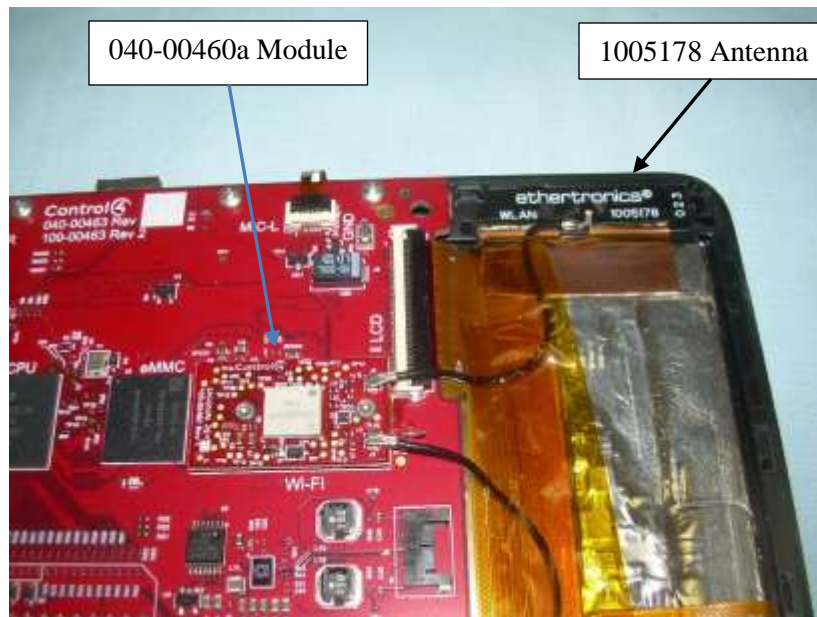
Photograph 18: 040-00460a Installed in C4-T4T8-XX with 1005178 Antenna Installed
