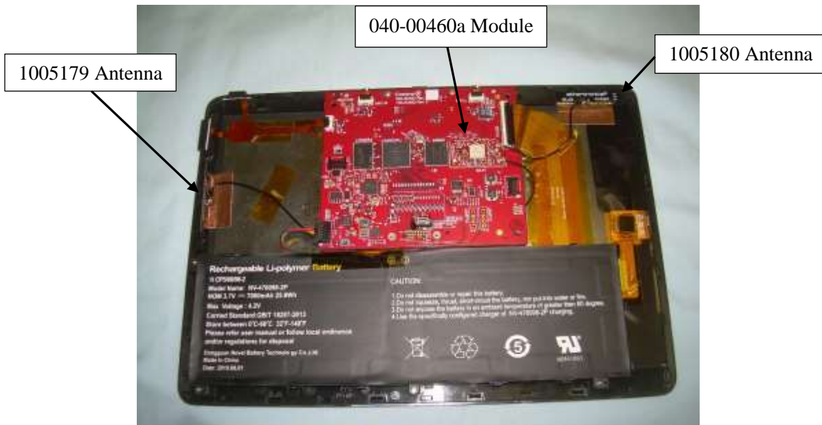
Photograph 15: 040-00460a Installed in C4-T4T10-xxwith 1005180 and 1005179 Antennas Installed
