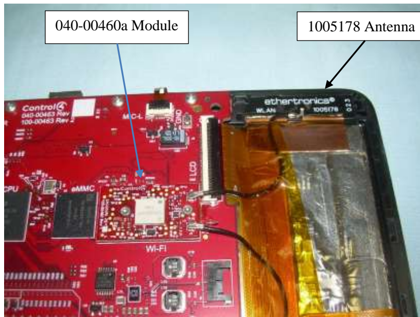
Photograph 19: 040-00460a Installed in C4-T4T8-XX with 1005178 Antenna Installed
