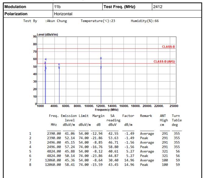
Note 1: Emission Level (dBuV/m) = SA Reading (dBuV) + Factor\* (dB/m)
