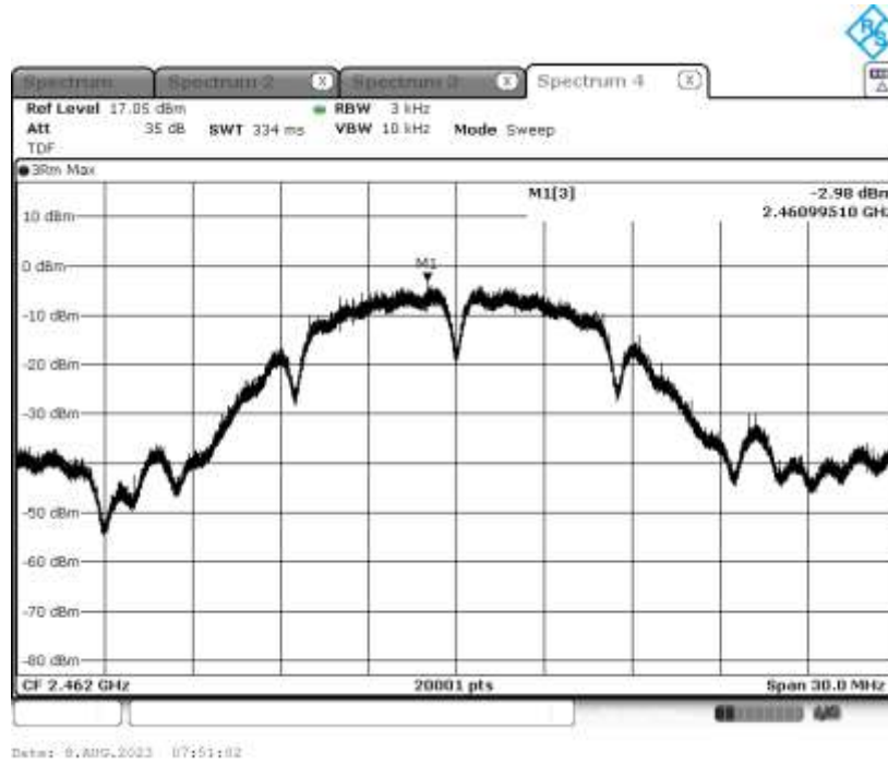
Graph 20: Highest Channel Output 3 kHz PSD Plot (Method AVGPSD-3)
