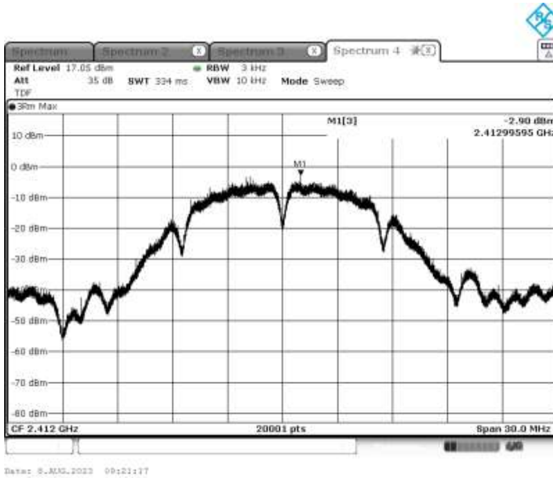
Graph 18: Lowest Channel 3 kHz PSD Plot (Method AVGPSD-3)
