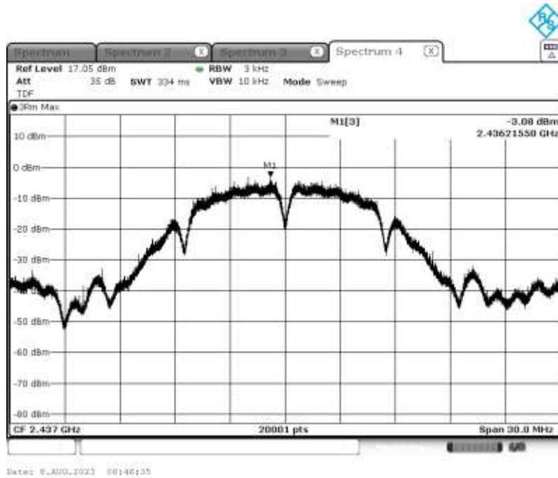
Graph 19: Middle Channel 3 kHz PSD Plot (Method AVGPSD-3)
