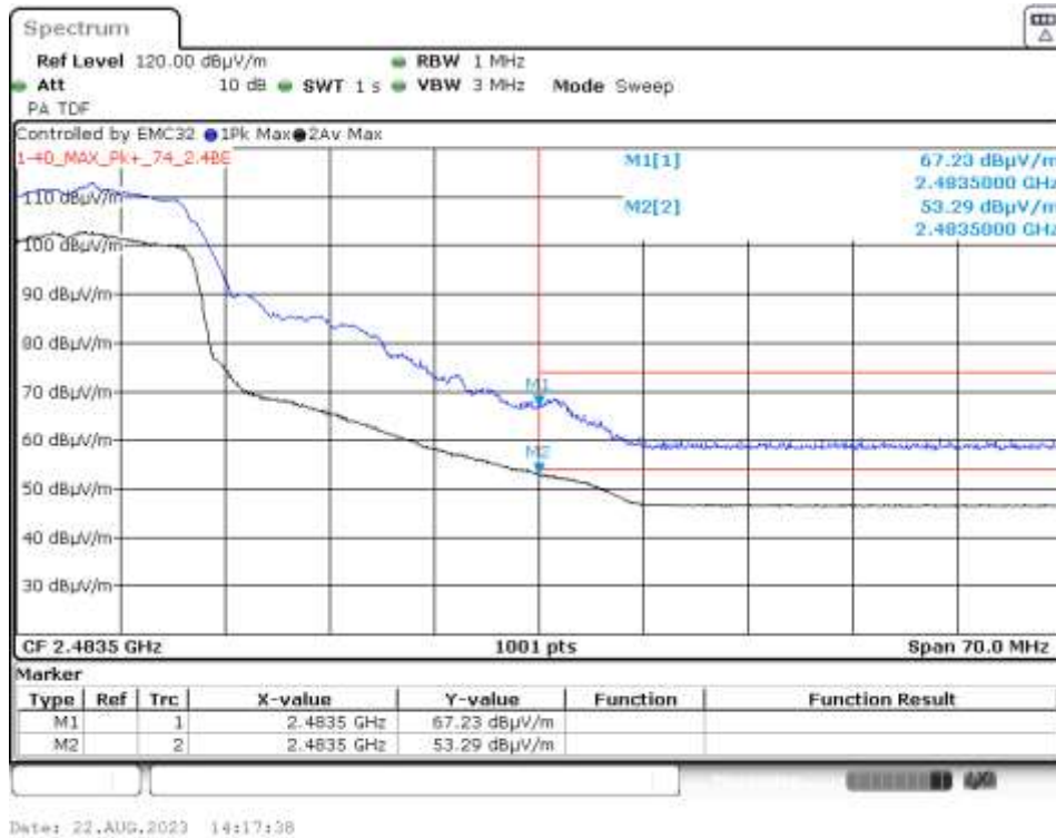
Graph 34: Radiated Upper Band Edge Plot (Transmitting 2452MHz, Power Level 17)
