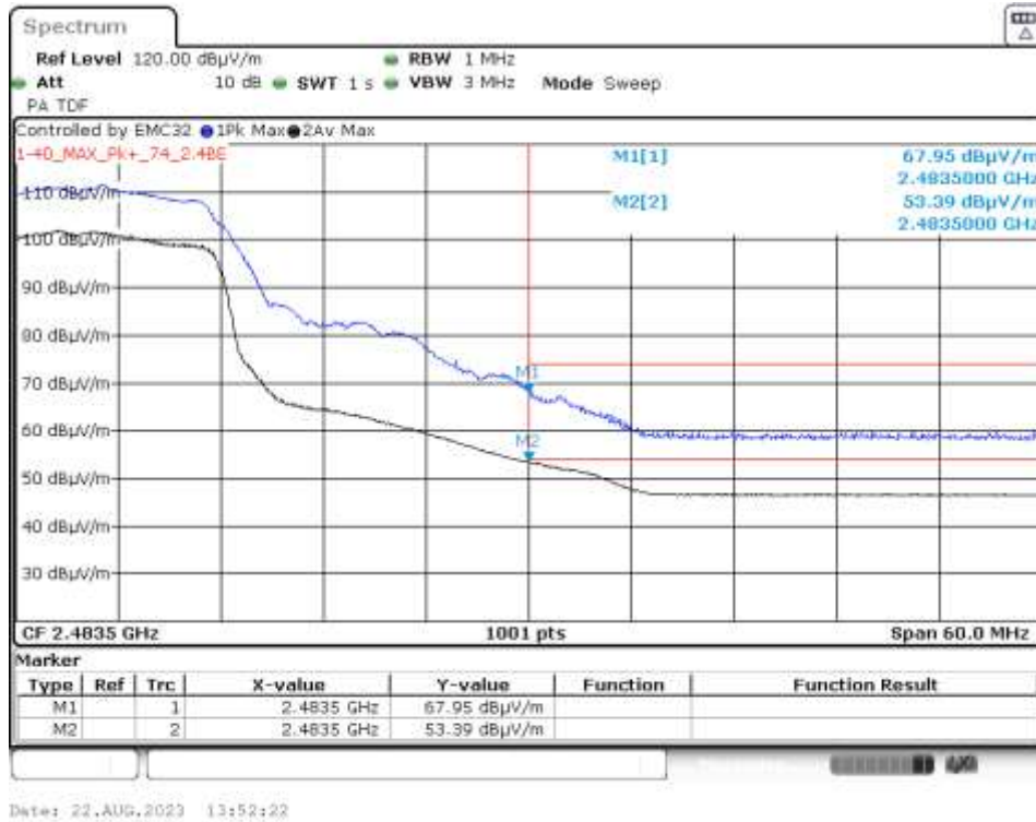
Graph 35: Radiated Upper Band Edge Plot (Transmitting 2457MHz, Power Level 16)
