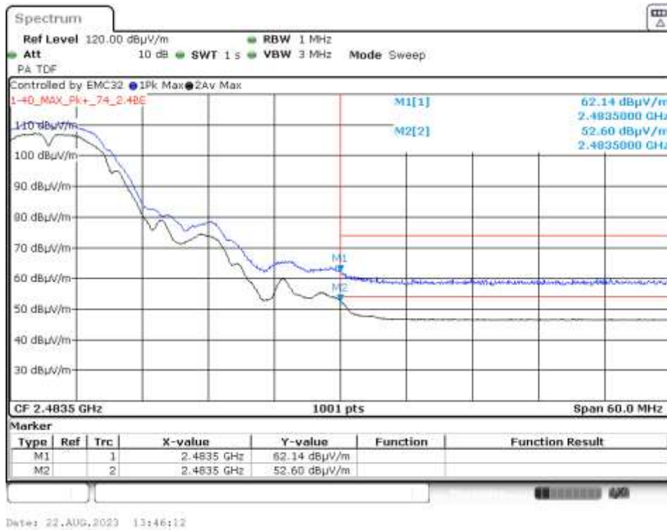
Graph 8: Radiated Lower Band Edge Plot (Transmitting 2417MHz, Power Level 20)
