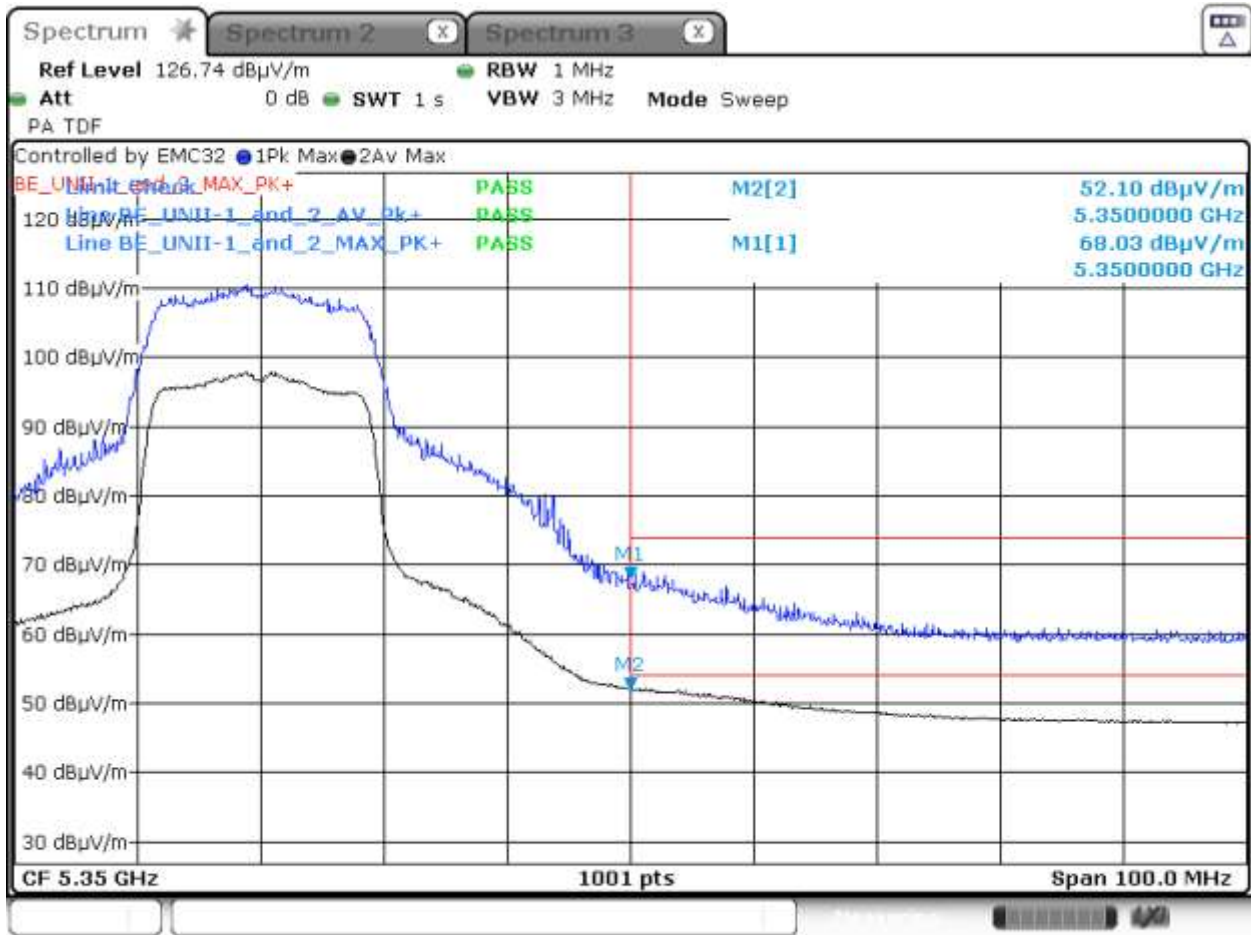
Graph 26: Radiated Restricted Band Edge Transmitting at 5320 MHz (Power Level 18, -1.9dB Margin)
