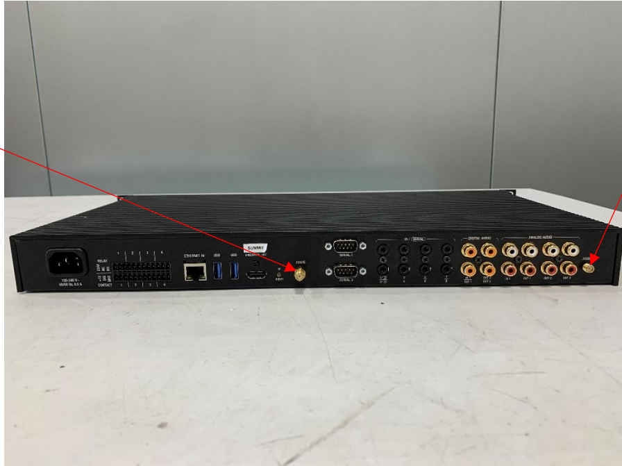
Photograph 5: Back View Showing All DUT Ports
